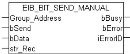
This function block sends a 1-bit EIB value to the parameterized group address. As entry value there is an EC61131-3 BOOL-Variable. The data is sent at a rising edge of *bSend*. As long as the block is active, the bit *bBusy* is set. *bBusy* is set back to FALSE if the EIB command is sent or an error occurs. An error is displayed by setting the variable *bError*. In this case the error code is given in *iErrorID*.
