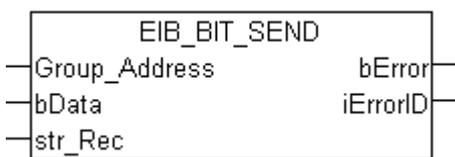
This function block sends a 1-bit EIB value to the set group address. An IEC61131-3 BOOL variable is available as input value. The data are only transferred if there is a change in the data value. If the value changes again within 200 milliseconds, new data are only sent to the EIB device after another 200 millisecond has passed (see diagram). No new EIB telegram is sent if the value changes within the "min. send time" but falls back to the old, already sent value within the "min. send time".
