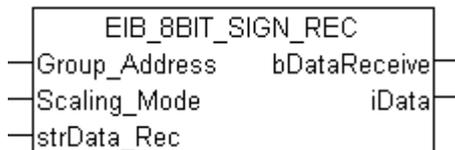
This function block receives 8 bits of EIB data on the set group address and converts them into an IEC61131-3 INT variable. In addition the value may be converted automatically.
