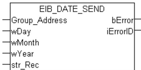
This function block sends a 3-byte EIB value to the set group address. Three IEC61131-3 word variables are available as input values. The data are sent when the block is called for the first time and then every 5 minutes.
