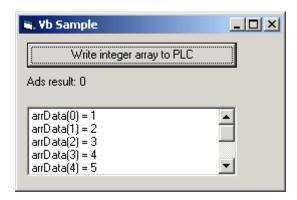
A connection to the PLC task of the BC9000 Bus Controller is established in the *Form\_Load* routine (port 800 and network address "172.16.17.63.1.1"). The first four digits of the network address correspond to the IP address of the bus controller. The desired service from the PLC task is encoded in the index group and index offset parameters. E.g.:
