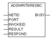
The ADSWRITERESBC function block is used to acknowledge indications of a PLC task. A response is sent to the ADS source device via a positive edge at the RESPOND input. The source device is addressed via the PORT and NETID parameters. The INVOKEID parameter is used by the source device to assign the responses to the requests and is adopted by the output of the <u>ADSWRITEIND [\* 17]</u> function block. An error code can be returned to the ADS source device via the RESULT parameter.
