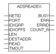
This function block allows execution of an ADS read command, to request data from an ADS device.
