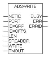
This function block permits execution of an ADS write command, for the transfer of data to an ADS device.
