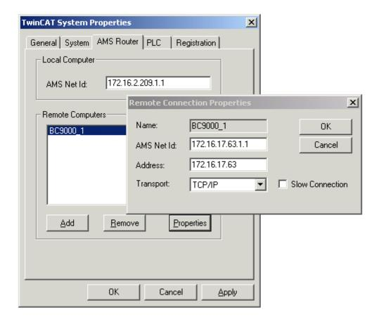
The TwinCAT system menu can be accessed by clicking the TwinCAT icon->properties in the taskbar. Select *Add* in the *AMS Router* tab. Enter an arbitrary name for the remote PC in the dialog. The network address is entered in *AMS Net Id.* It consists of the IP address of the BC9000 and two further digits: "1.1". The IP address of the BC9000 is entered again in *Address*. The IP address must correspond to the address that was set via the dip switches on the bus controller.
