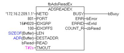
In this sample, an ADS read command is sent to an ADS device with network address '172.16.2.209.1.1' and port number 801. This port number could, for instance, be used to address the PLC's first runtime system. The service to be executed is encoded in the index group and the index offset parameters. Here, 10 bytes of PLC variable data in the flags area are to be read starting from byte offset 100. If successful, 10 bytes of data are copied to the address of the *Buffer* variable.
