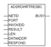
The ADSRDWRTRESBC function block is used to acknowledge indications of a PLC task. A response is sent to the ADS source device via a positive edge at the RESPOND input. The source device is addressed via the PORT and NETID parameters. The INVOKEID parameter is used by the source device to assign the responses to the requests and is adopted by the output of the <u>ADSRDWRTIND</u> [• 20] function block. An error code can be returned to the ADS source device via the RESULT parameter.
