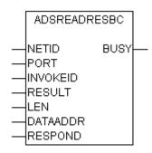
The ADSREADRESBC function block is used to acknowledge READ indications of a PLC task. A response is sent to the ADS source device via a positive edge at the RESPOND input. The source device is addressed via the PORT and NETID parameters. The INVOKEID parameter is used by the source device to assign the responses to the requests and is adopted by the output of the <u>ADSREADIND</u> [• 17] function block. An error code can be returned to the ADS source device via the RESULT parameter.
