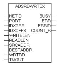
This function block allows execution of a combined ADS write/read instruction. Data is transmitted to an ADS device (write) and its response data read with one call.
