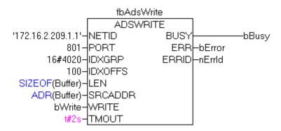
In this sample, an ADS command is sent to an ADS device with network address '172.16.2.209.1.1' and port number 801. This port number could, for instance, be used to address the PLC's first runtime system. The service to be executed is encoded in the index group and the index offset parameters. If successful, 10 bytes of data (*Buffer* variable) are written into the flags area of the target device, starting at byte offset 100.
