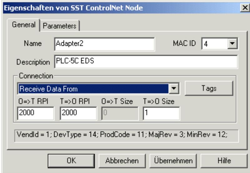
It is also possible for the Consume Buffer-ID to be set, under parameters. This must agree with the Produce Buffer ID set in the PLC 5.
