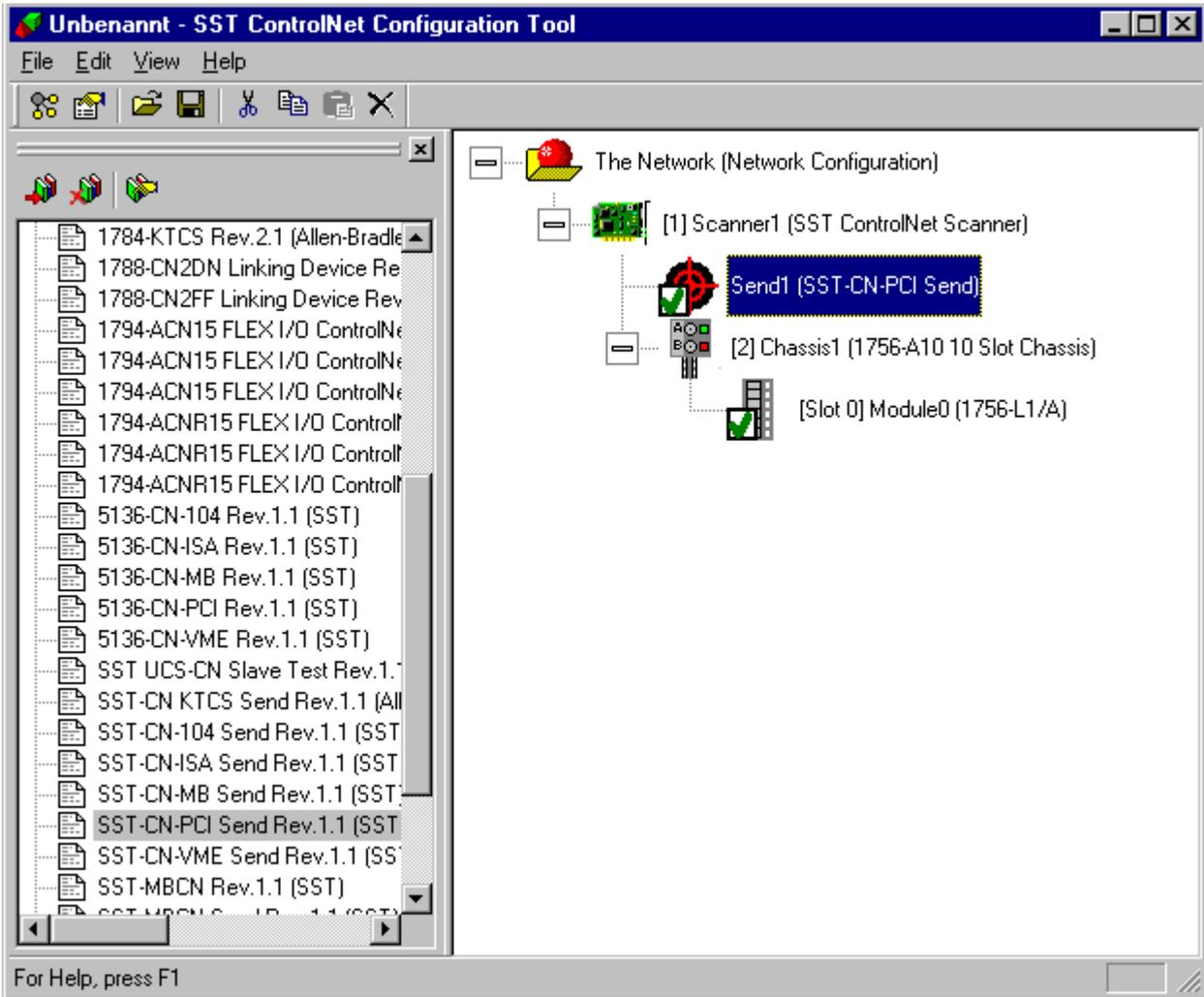
Double-clicking on the send connection that has been inserted brings up a dialog in which the T=>O Size (outputs, Control-Logix receive data (Consumed must be selected for the corresponding tag), is set.
