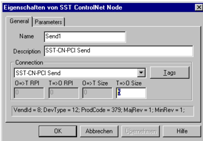
It is also possible for the Produce Buffer ID to be set, under parameters. This must agree with the instance of the input tag set in the Control-Logix. **This Produce Buffer ID is also used for addressing the process data from TwinCAT (-> [Process data](#) |> [27](#)) send connection):**
