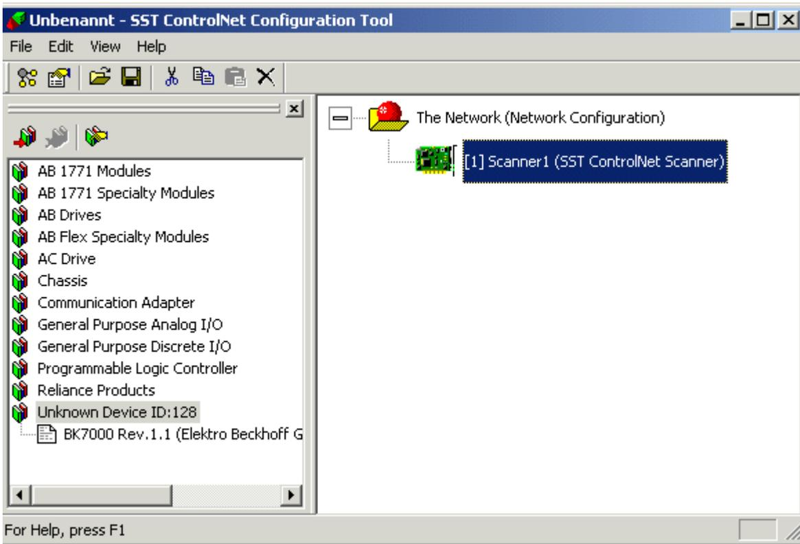
The scanner's properties can be set by double-clicking on it. As a rule, only the card concerned must be entered under "Card Name", along with the Mac-ID if appropriate.
