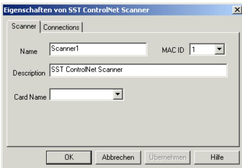
ControlNet devices can now be dragged to the scanner from the EDS library using the left mouse button.
