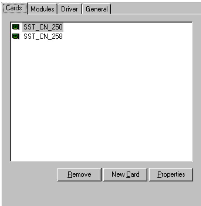
One entry should be deleted (using the Remove button), and the other should be edited (using Properties). A new dialog appears in which the I/O address of the 5136-CN is to be set in accordance with the DIP switch and where the memory address and the name can be adjusted.
