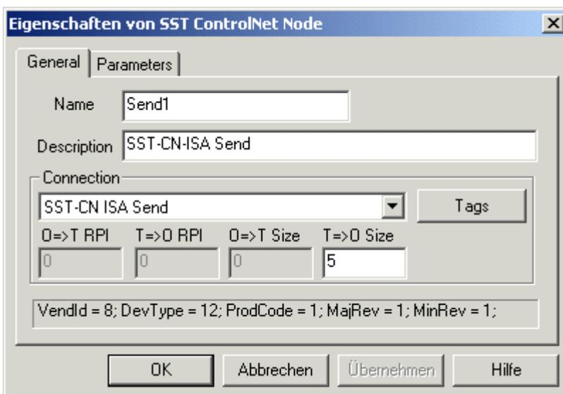
It is also possible for the Produce Buffer ID to be set, under parameters. This must agree with the Consume Buffer ID set in the PLC 5. **This Produce Buffer ID is also used for addressing the process data from TwinCAT (-> [Process data](#) |> 27) send connection)**
