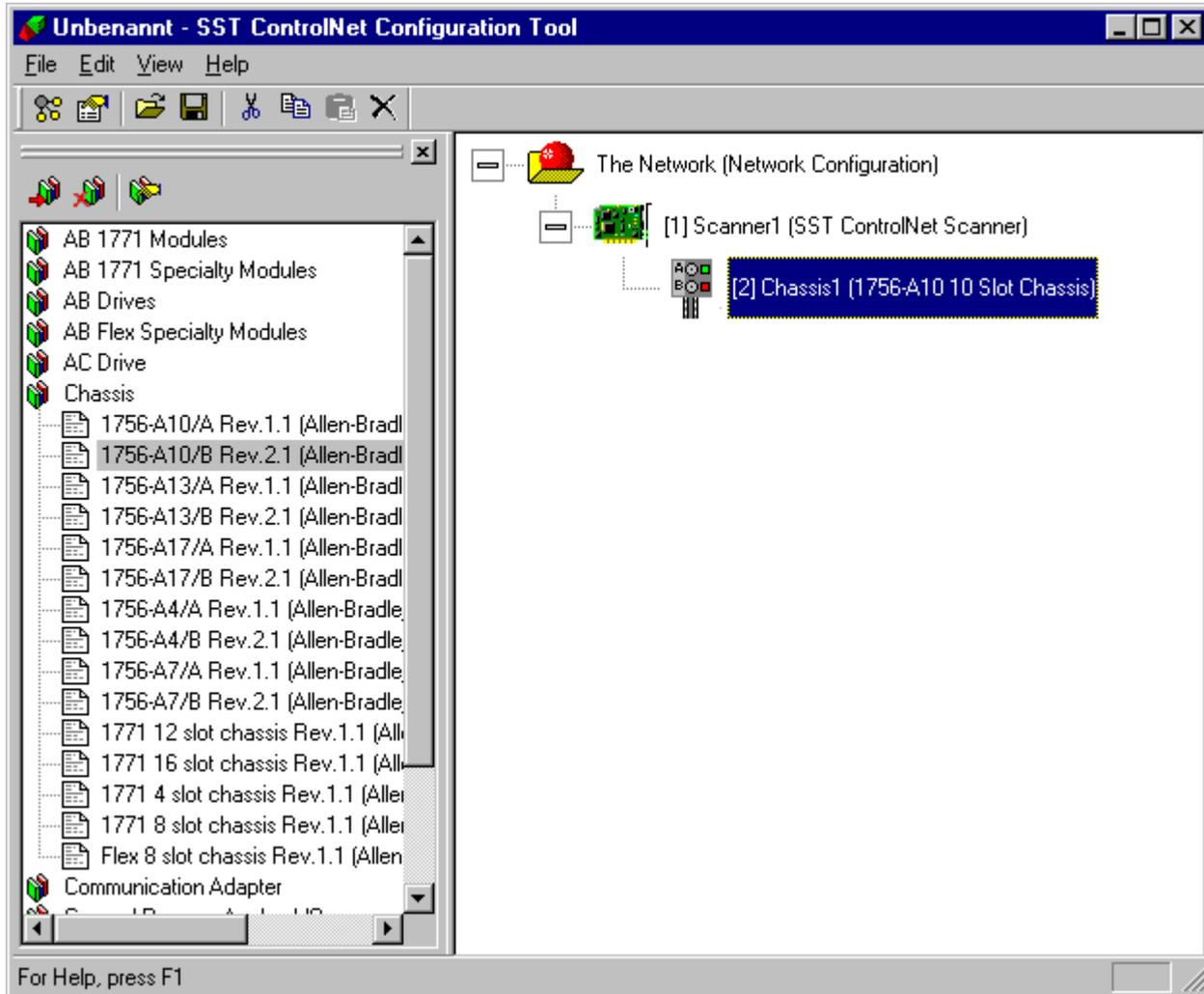
The appropriate Control-Logix CPU is to be dragged with the left mouse button from the "Programmable Logic Controller" entry across to the chassis in the right-hand window. The slot number of the CPU (not of the ControlNet interface) must be selected here. The Control-Logix CPU then appears in the right-hand window.
