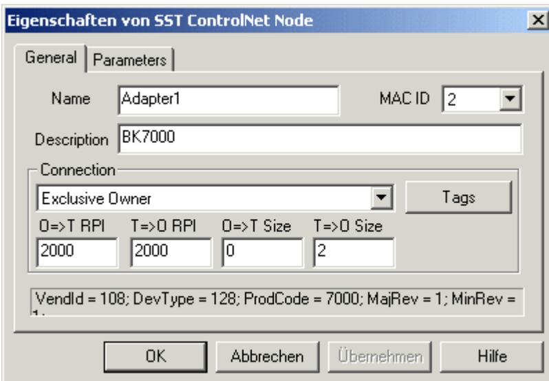
The "O=>T Size" (the length of the output in words) and the "T=>O Size" (the length of the input in words + 2) are to be set in the dialog in accordance with the terminal configuration. In order to calculate the output and input lengths, the BK7000 supports four mapping schemes, which are set automatically in accordance with the selected size:
