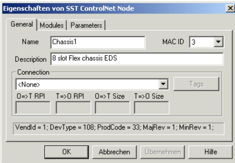
Double-clicking the Flex I/O adapter allows the "O=>T RPI" or "T=>O RPI" values to be set. These values must be greater than or equal to the network settings for the NUT interval.
