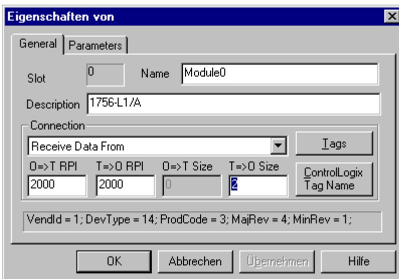
Under the "Control Logix Tag Name" button it is still necessary for the tag name of the corresponding Control-Logix output tag to be stated.
