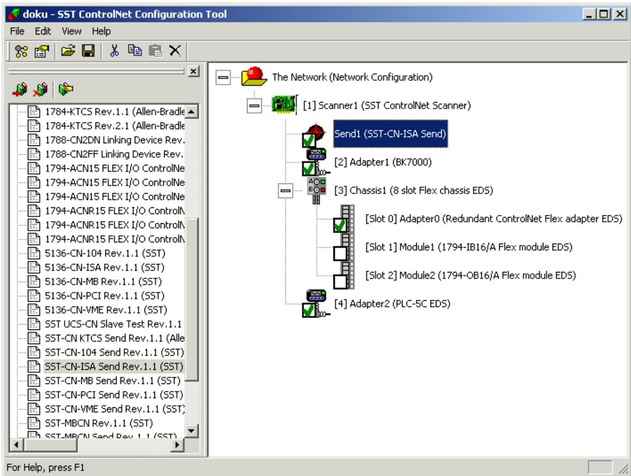
Double-clicking on the send connection that has been inserted brings up a dialog in which the T=>O Size (outputs, PLC 5 receive data), is set.
