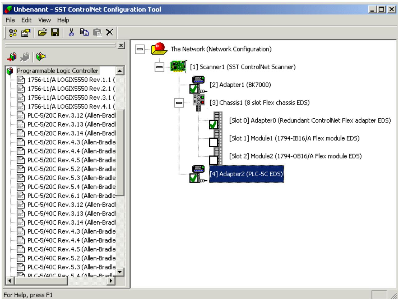
A double-click on the PLC 5 will bring up a dialog in which the "T=>O Size" (inputs, PLC 5 send data) in Words and, when appropriate, the Mac-ID and the "O=>T RPI" or the "T=>O RPI" can be set. These values must be greater than or equal to the network settings for the NUT interval.
