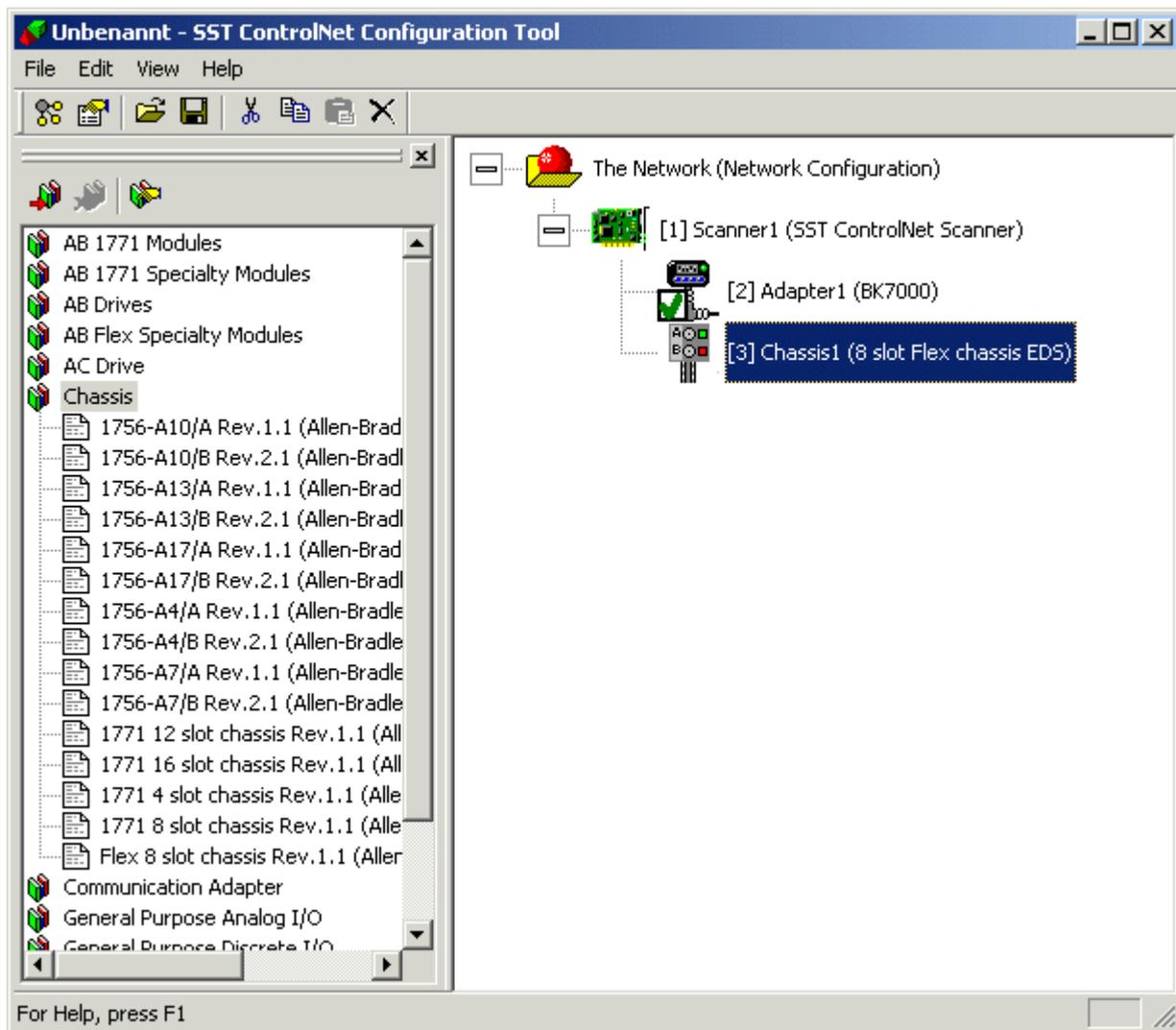
Next, the corresponding Flex I/O adapter is to be dragged with the left mouse button from the EDS library's "Communication Adapter" entry, across to the chassis in the right hand window - a field appears with 0 for the slot number, which is to be selected. The Flex-I/O adapter then appears in the right hand window.
