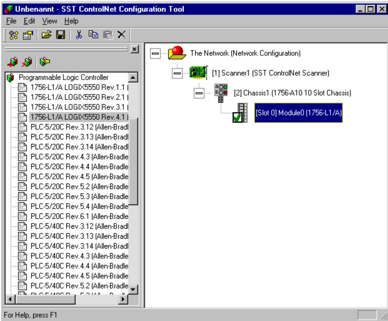
A double-click on the Control-Logix CPU will bring up a dialog in which the "T=>O Size" (inputs, Control-Logix send data (Producer must be clicked on the corresponding tag)) in Words and, when appropriate, the Mac-ID and the "O=>T RPI" or the "T=>O RPI" can be set. These values must be greater than or equal to the network settings for the NUT interval.
