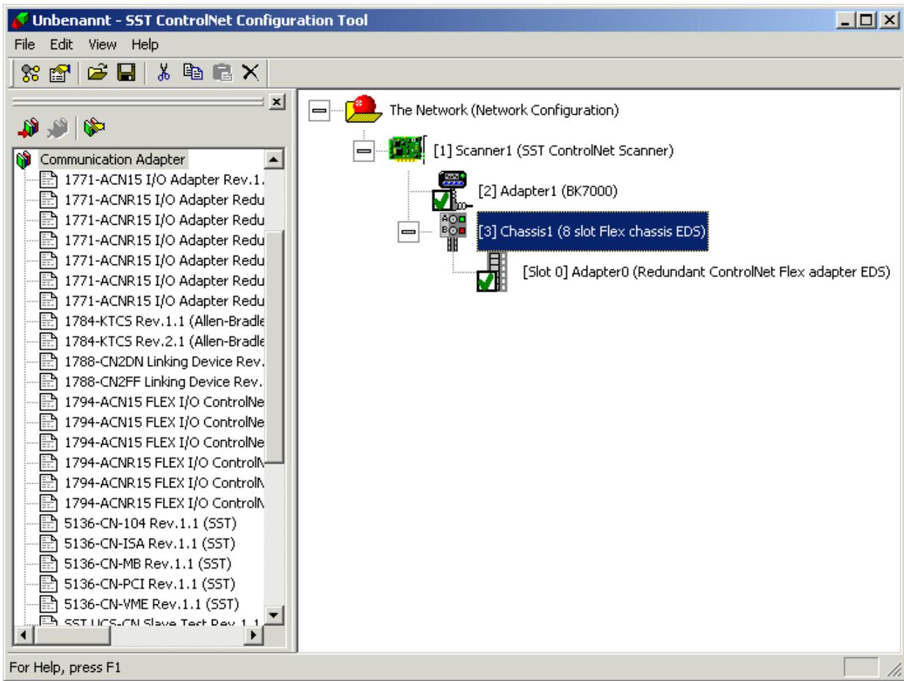
It is finally necessary for the appropriate modules for the Flex-I/O device to be added by dragging them with the left mouse button from the "General Purpose Analog IO" or "General Purpose Digital IO" entries, across to the chassis in the right-hand window. A field with the slot number, which has to be selected, appears.
