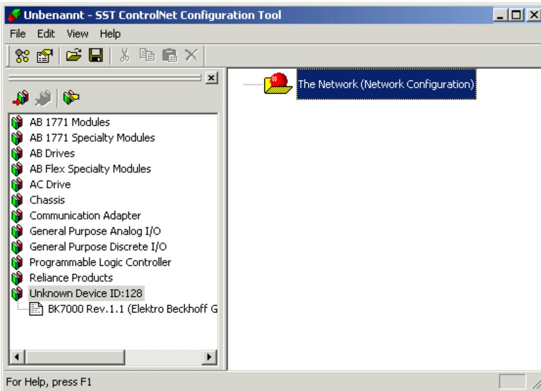
The 5136-CN PC card is first entered as the scanner. This is achieved by clicking on "The Network (Network Configuration)" with the right mouse button and selecting "New Scanner".
