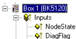
For each CANopen fieldbus node there is a node state input variable, which signals the status of the current slave during the running time and can be linked, for example with the PLC.
