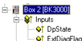
Each Profibus slave box contains two diagnostic input bytes which signal the state of each slave during the running time, and which can be linked, for example with the PLC.
