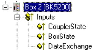
Each DeviceNet fieldbus node contains one diagnostic input byte which signals the status of the current slave during the running time and can be linked, for example with the PLC.
