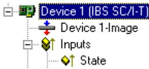
The IBS ISA SC-I/T automatically provides two input words whose bits describe the status of the card and the Interbus:
