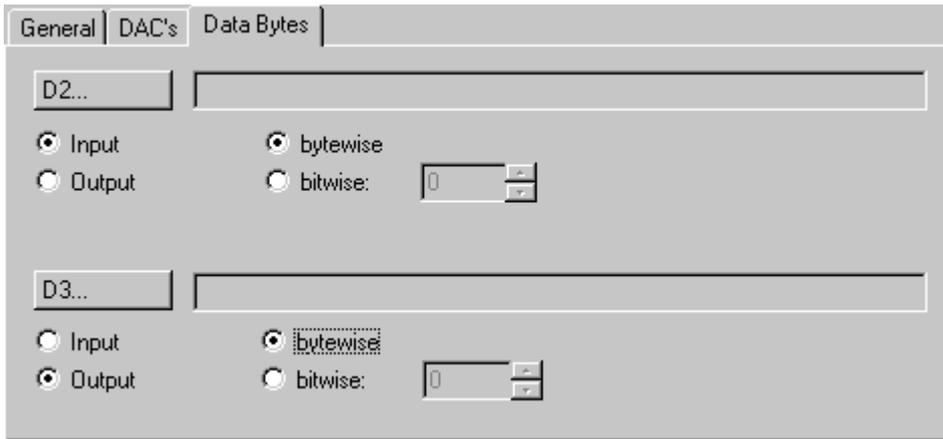
**D 2...:** Opens the link dialogue for the first data byte (D2 in the telegram).
