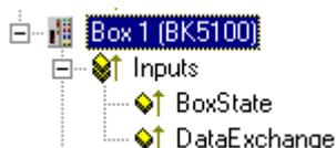
For each CANopen fieldbus node there is a box state input variable, which signals the status of the current slave during the running time and can be linked, for example with the PLC.
