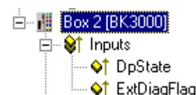
Each Profibus slave box contains two diagnostic input bytes which signal the state of each slave during the running time, and which can be linked, for example with the PLC.
