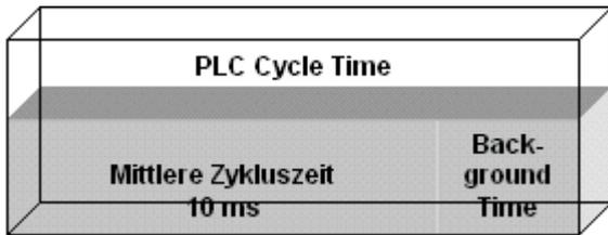
PLC cycle time = mean cycle time + 20% = 10 ms + 20% = 12 ms
