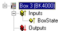
Each InterBus-S box contains one diagnostic input byte which signals the status of the current slave during the running time and can be linked, for example with the PLC.
