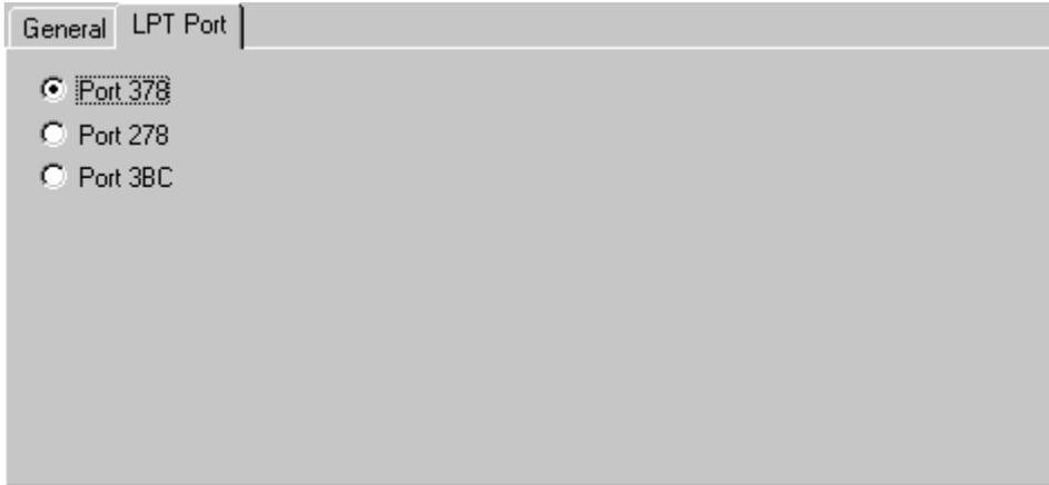
There are three port address options. These echo the standard PC interfaces LPT1, LPT2 and LPT3. Your PC manual will tell you which LPT port on your computer corresponds to which port address. Alternatively check the current BIOS setting.
