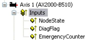
The diagnosis [Inputs \[▸ 178\]](#) of an AX2000-B510 don't differ from the diagnosis inputs of other TwinCAT CANopen nodes (see also: "[FC510x: Box-Diagnosis \[▸ 177\]](#)").
