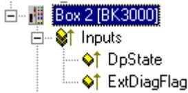
Each Profibus slave fieldbus box contains two diagnostic input bytes which signal the state of each slave during the running time and which can be linked, for example with the PLC.
