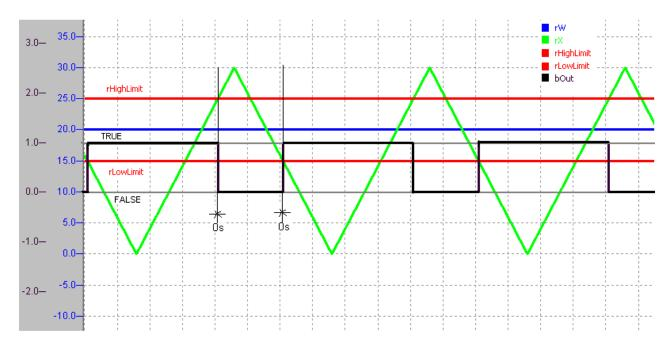
Figure: FB\_HVAC2PointCtrl timing diagram
