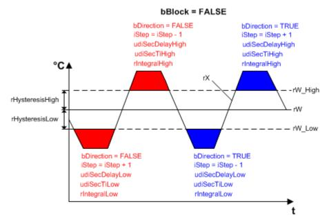
Fig. 13: FB\_HVACI\_CtrlStepParameter
