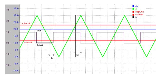
Figure: FB\_HVAC2PointCtrl timing diagram
