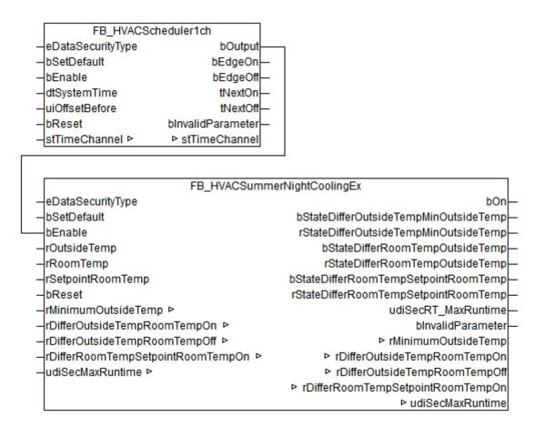
**rOutsideTemp:** input for the outside temperature.
