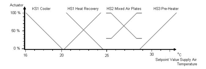
**Example:** Supply air temperature regulation in an air conditioning system with an air cooler, a heat recovery unit, a mixed air chamber and an air heater, as shown in the figure above.
