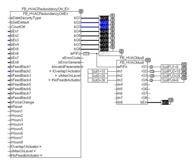
There are 4 drives with speed controllers (SetFC1 – SetFC4), of which a maximum of three should be running. The control range of 0 to 300% is divided into 3 setpoints (Set1 to Set3). The output *arrFiFo* of *FB\_HVACRedundancyCtrlEx* supplies *FB\_HVACMux8* with the assignment description. In the sample the array contains: 2,3,0,0,0,0,0,0. Therefore Q2 was switched on first and then Q3. As a result *rln1* is now output on *rQ2* and *rln2* on *rQ3* in *FB\_HVACMux8*.
