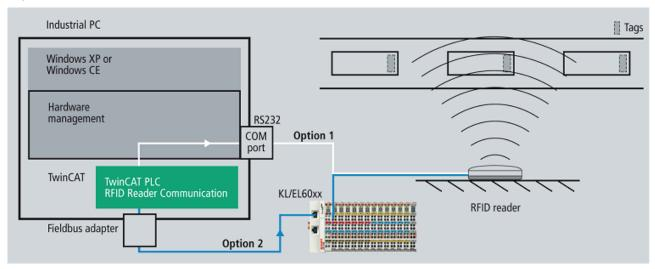
Schematic diagram of an RFID reader connection [▶ 14]
