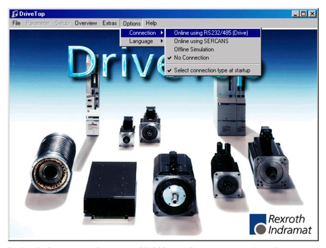
The DriveTopServer searches for disposable SERCOS drives, if the connection is available. The corresponding device is then selectable in the case of the DriveTop.
