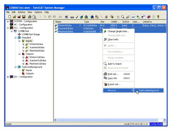
Since the task's cycle time determines the update cycle on the I/O bus, it is essential that the data structures for communication between the fast communication task and the hardware be assigned to that task. The corresponding entries under the standard task's inputs and outputs are dragged with the mouse or with the *Move to* context menu into the communication task.
