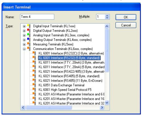
Then the input and output data are individually linked to the corresponding PLC variables (of types <u>KL6inData5B</u> [▶ 36] and <u>KL6outData5B</u> [▶ 36]).
