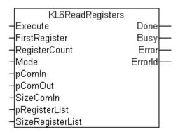
The KL6ReadRegisters function block reads one or several registers of a KL6xxx serial Bus Terminal.
