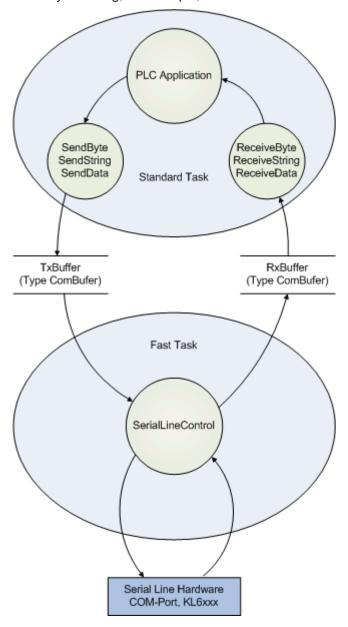
Data buffers of type ComBuffer [> 34] are used to decouple the different speeds of the fast communication task and the standard task. They are written and read asynchronously.
