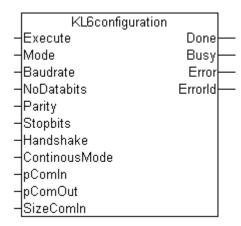
The KL6configuration function block initialises and configures a KL6xxx Serial Bus Terminal.
