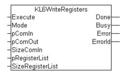
The function block KL6WriteRegisters writes data to one or several registers of a serial KL6xxx Bus Terminal.
