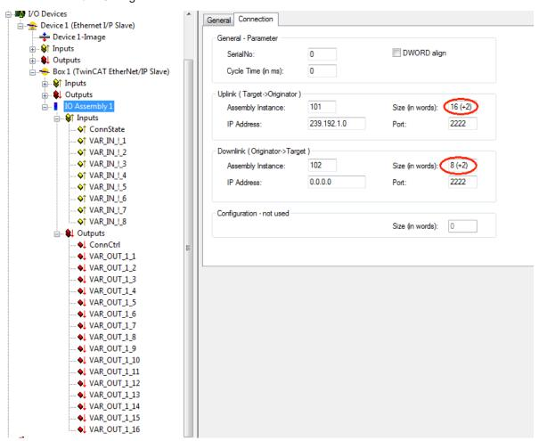
10. The Pre-Configuration of TwinCAT EtherNet/IP Slave is finished now. Activate the configuration and go on with Integration in RSLogix5000.
