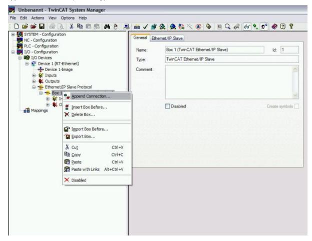
7. Depending on application requirements it's possible to define the size of Processdata Image separately for inputs and outputs from 1 up to 502 bytes. Please find an example for defining 8 Word Input Processdata as shown below.
