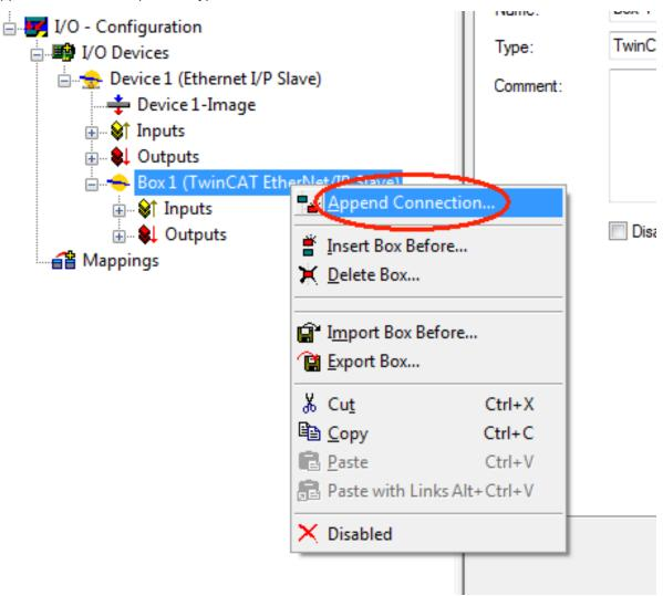
8. Depending on application requirements it's possible to define the size of Processdata Image separately for inputs and outputs from 1 up to 502 bytes. Please find an example for defining 8 Word Input Processdata as shown below.
