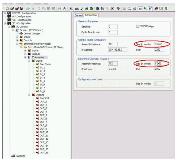
9. The Pre-Configuration of TwinCAT EtherNet/IP Slave is finished now. Activate the configuration and go on with Integration in RSLogix5000.
