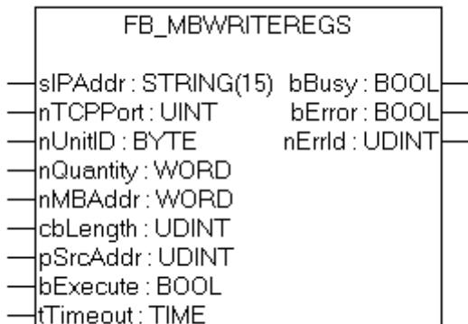
This function is used for writing 1 to 128 output registers (16 bit).
