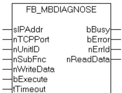
The diagnosis function provides a series of tests for checking the communication system between the master and the slave and for examining a variety of internal error states within the slave.
