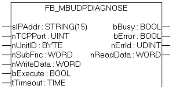
The diagnosis function provides a series of tests for checking the communication system between the master and the slave and for examining a variety of internal error states within the slave.
