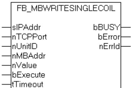
This function is used for writing a single digital output (coil). Bit access is used.
