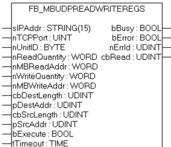
This function first reads 1 to 128 output registers (16 bit) and then writes 1 to 128 output registers (16 bit).
