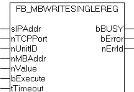
This function is used for writing an individual output register. 16 bit access is used.
