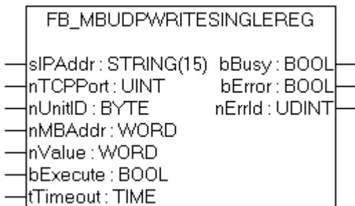
This function is used for writing an individual output register. 16 bit access is used.
