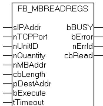
This function is used for reading 1 to 128 output registers (16 bit). The first byte contains the lower eight bits and the second byte the upper eight bits.
