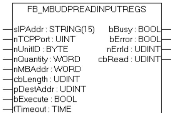
This function is used for reading 1 to 128 input registers (16 bit). Endian
