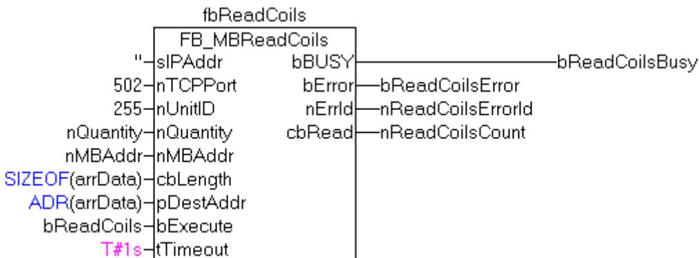
After a rising edge of "bExecute" and successful execution of the ReadCoils command, the content of digital outputs 6 - 15 is written into the arrData array:
