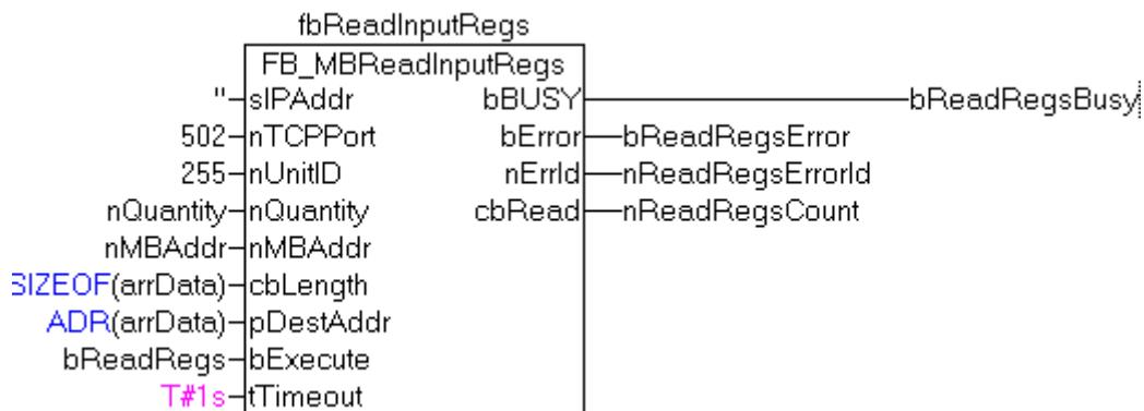
After a rising edge of "bExecute" and successful execution of the ReadRegs command, the content of registers 3-5 is in the arrData array:
