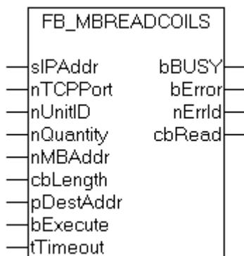
This function is used for reading 1 to 2048 digital outputs (coils). One digital output corresponds to one bit of the read data bytes.
