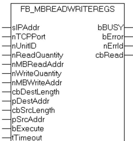
This function first reads 1 to 128 output registers (16 bit) and then writes 1 to 128 output registers (16 bit).
