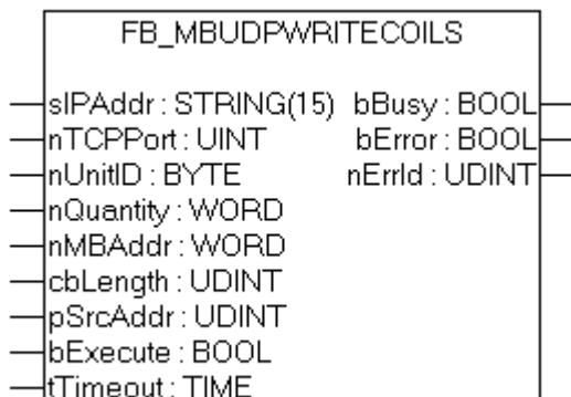
This function is used for writing 1 to 2048 digital outputs (coils). One digital output corresponds to one bit of the write data bytes.
