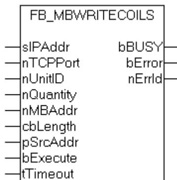
This function is used for writing 1 to 2048 digital outputs (coils). One digital output corresponds to one bit of the write data bytes.
