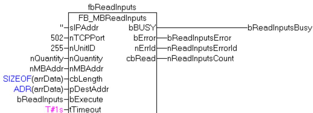
After a rising edge of "bExecute" and successful execution of the ReadInputs command, the content of digital inputs 30 - 49 is written into the arrData array:
