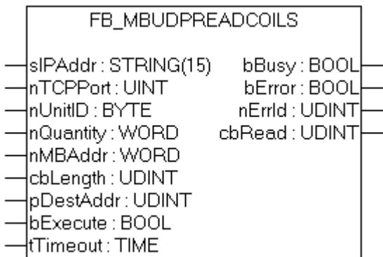
This function is used for reading 1 to 2048 digital outputs (coils). One digital output corresponds to one bit of the read data bytes.
