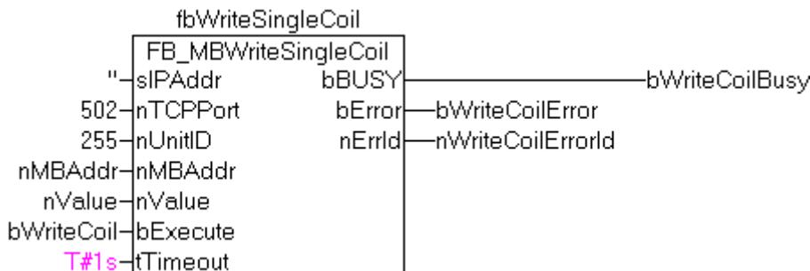
After a rising edge of "bExecute" and successful execution of the WriteSingleCoil command, digital output 4 is switched on.
