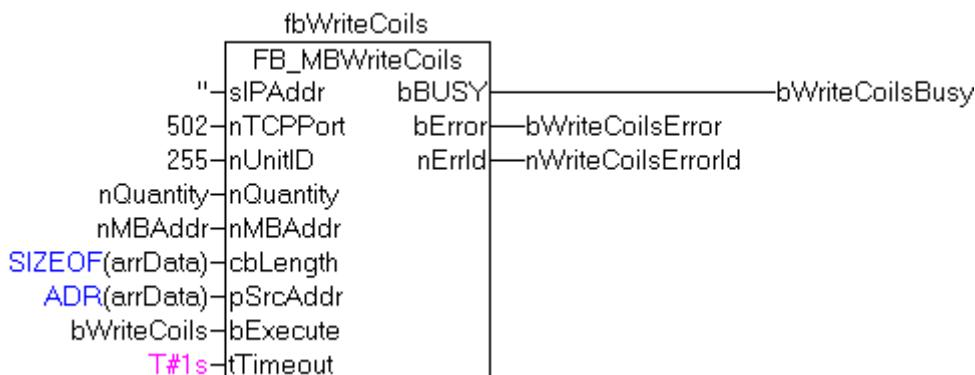
After a rising edge of "bExecute" and successful execution of the ReadCoils command, the content of the arrData array is written to digital outputs 15 - 24:
