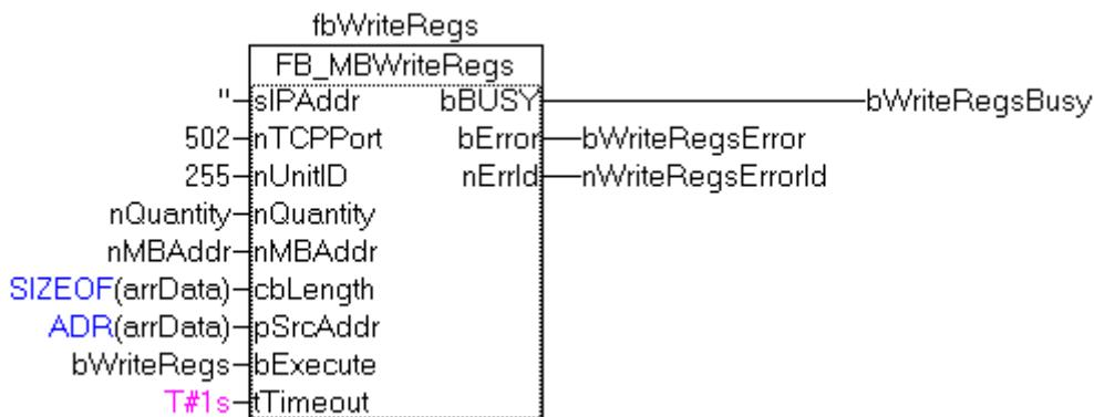
After a rising edge of "bExecute" and successful execution of the ReadRegs command, the content of the arrData array is written to registers 5-7.
