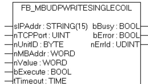
This function is used for writing a single digital output (coil). Bit access is used.
