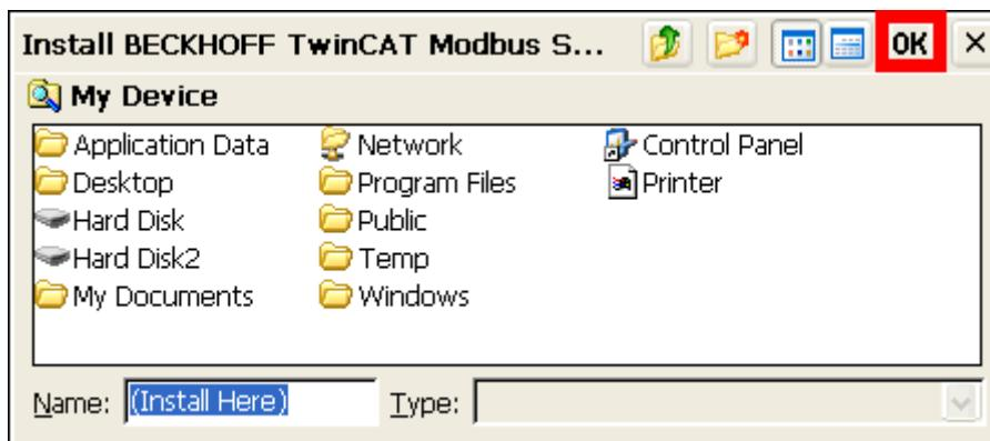
**Note:** The installer selects as target folder /Hard Disk/System by default.
