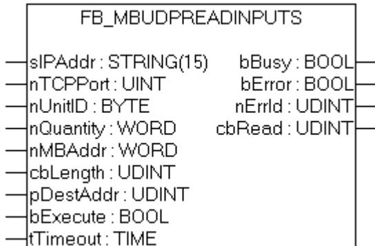
This function is used for reading 1 to 2048 digital inputs. One digital input corresponds to one bit of the read data bytes.
