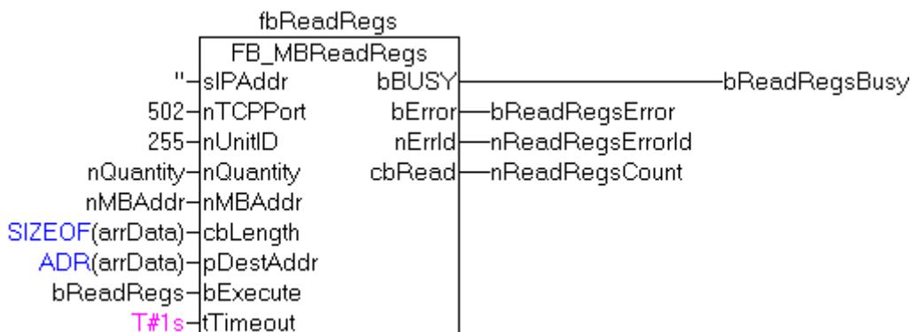
After a rising edge of "bExecute" and successful execution of the ReadRegs command, the content of registers 25 and 26 is in the arrData array:
