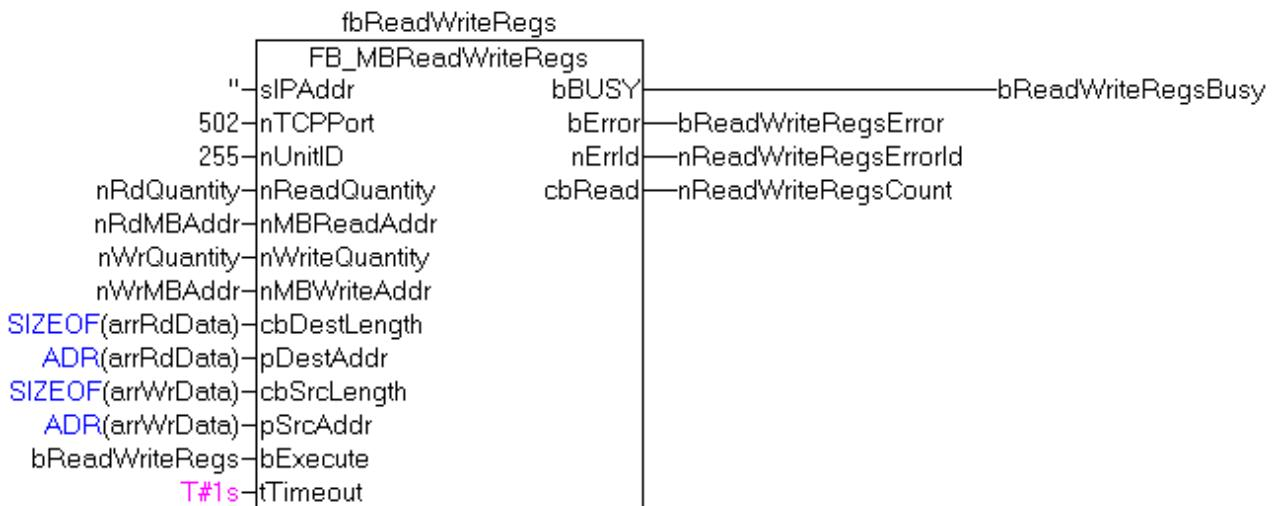
After a rising edge of "bExecute" and successful execution of the ReadWriteRegs command, arrRdData contains the read register data, and the data from arrWrData are written to the registers.
