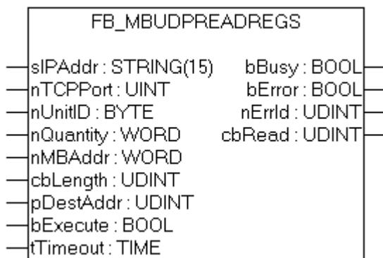
This function is used for reading 1 to 128 output registers (16 bit). The first byte contains the lower eight bits and the second byte the upper eight bits.
