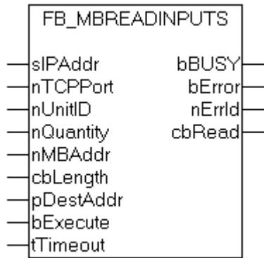
This function is used for reading 1 to 2048 digital inputs. One digital input corresponds to one bit of the read data bytes.
