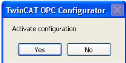
After selecting "Yes" this current configuration will be the start-configuration of the opc-server. With next start of OPC-Server this new configuration will be active.
