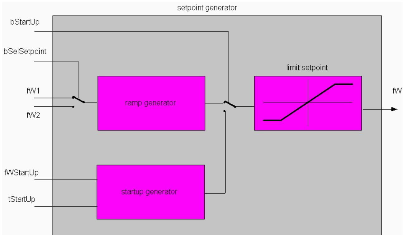
In order to permit "heater baking", a soft start can be parameterized. In this case, the temperature is first ramped up from ambient to a low setpoint ( $fW_{StartUp}$ ). This temperature is then maintained for a period of time ( $t_{StartUp}$ ), and only after that has elapsed does the ramp up to the actual setpoint begin.
