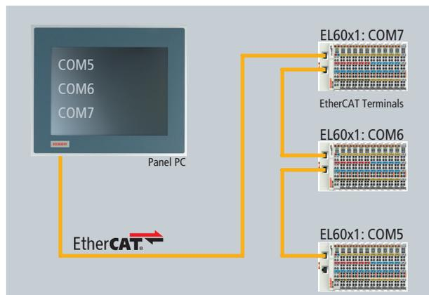
Fig. 1 Serial interface in the field
