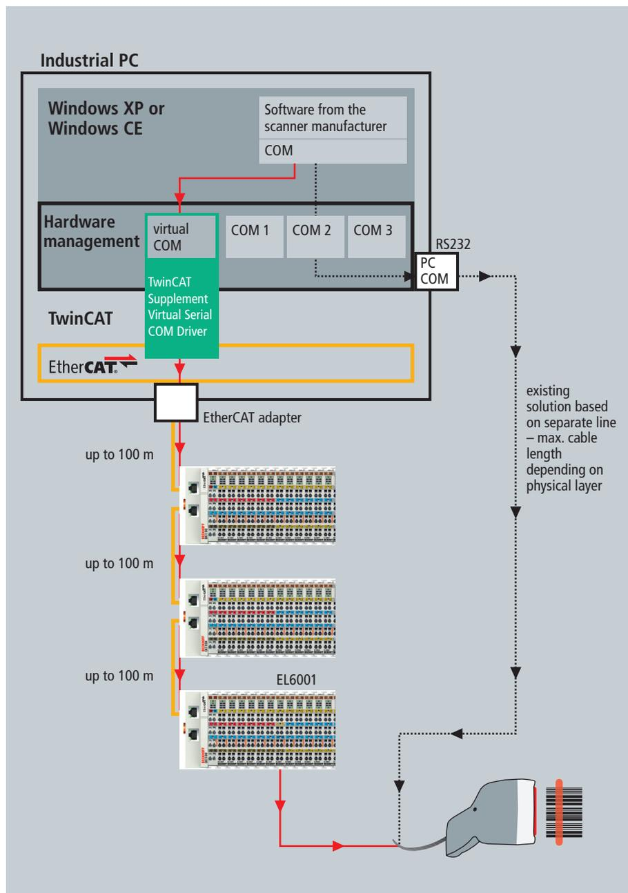
Fig. 2 Connecting a scanner
