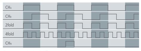
Fig. 1 Encoder signals with different resolutions
