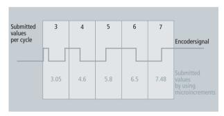
Fig. 3 Different encoder signals resolutions (with and without microincrements)
