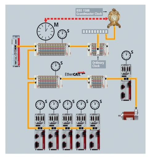
Fig. 2 Local clock generators in the field
