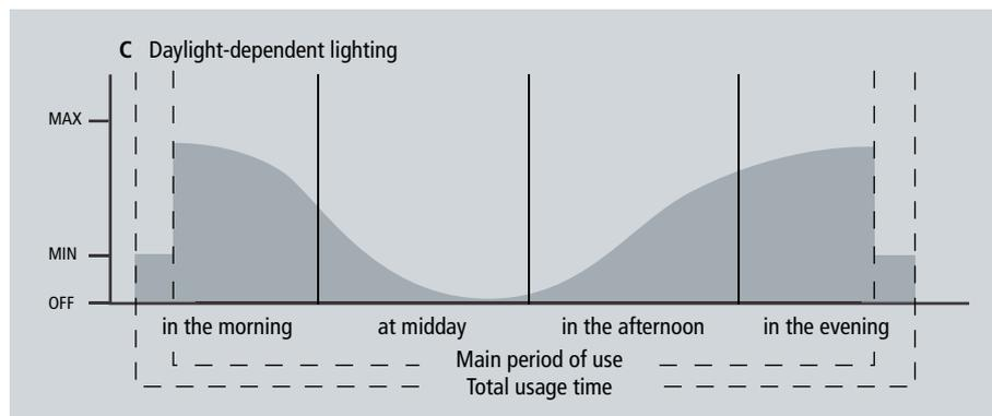
Fig. 5 Energy saving by means of central switching off, time-dependent and daylight-dependent lighting
