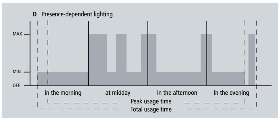
Fig. 6 Energy saving by means of presence-oriented lighting
