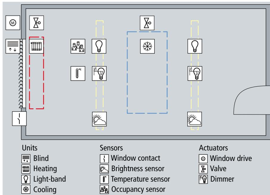
Fig. 4 Units, sensors and actuators for the control of an office
