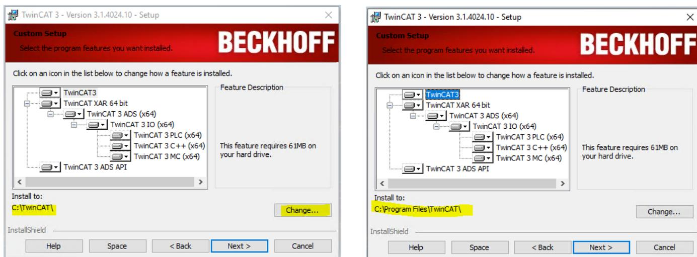
Please mind that already installed projects underneath C:\TwinCAT need to be moved. It is recommended to perform a backup of the complete device before such action. For security reasons, please remove the former content of C:\TwinCAT at the end of this sequence. This will also prevent confusion.
