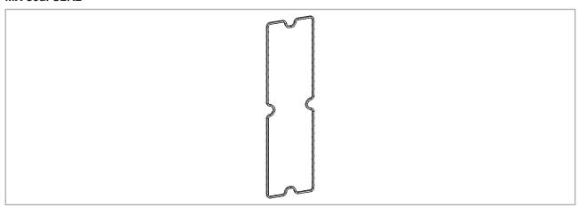
The S2R2 seal is available to replace worn and damaged seals on a 2-row MX module with two slots.
