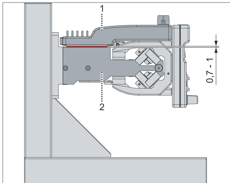
The air gap between the mounted NCT electronics [1] and the motor module [2] is preset to 1 mm ex factory. The air gap may be reduced to a minimum of 0.7 mm.
