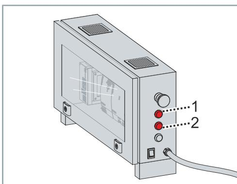
The *Stop button* [1] on the control cabinet must flash red.
