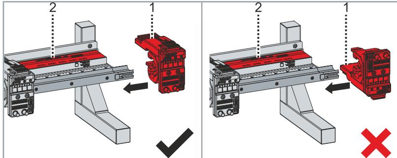
The NCT electronics [1] must be located on the side of the name plate [2] when the mover is inserted.
