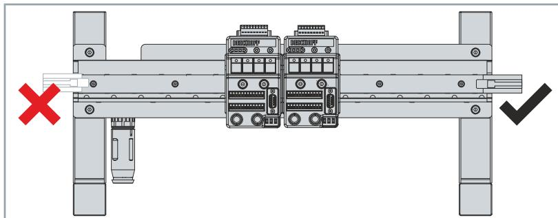
The rail on support may only be mounted on the motor module without connectors.
