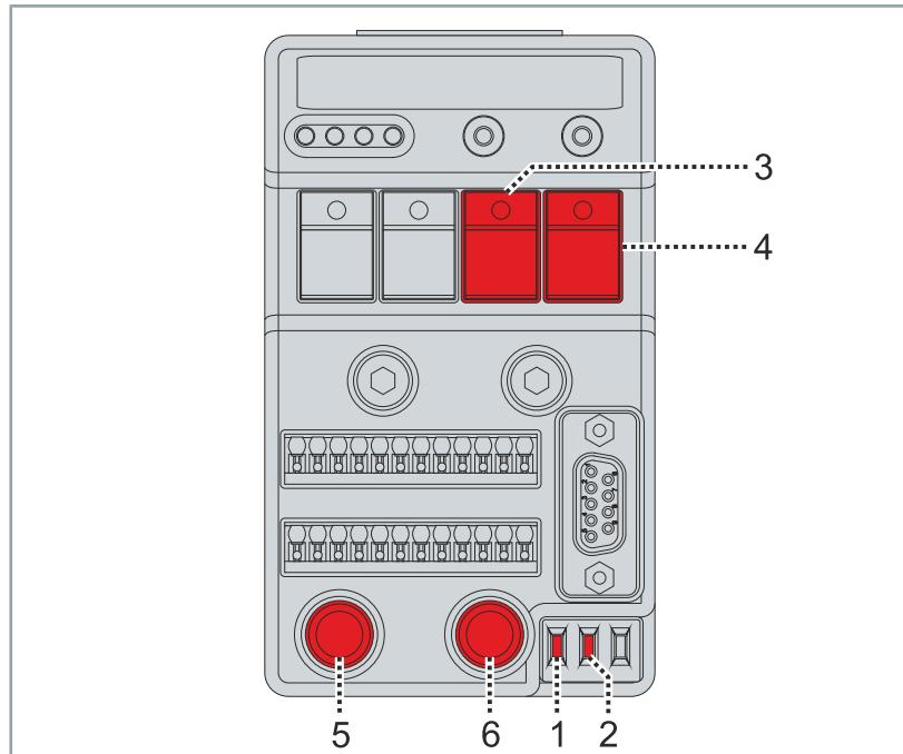
The position of the switches [1] and [2] on the test board determines whether the digital inputs [3] and [4] or the analog inputs [5] and [6] are enabled.
