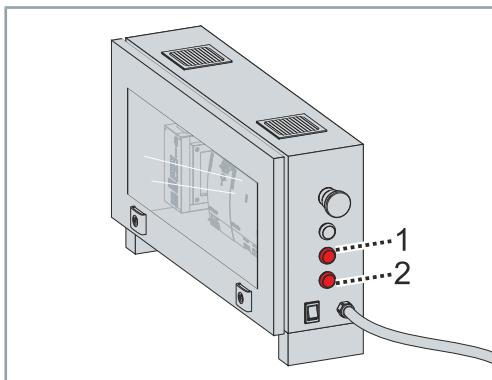
The *Stop* button [1] must light up red continuously.
