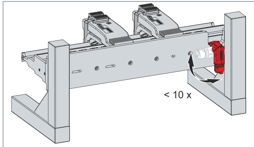
The connector of the module may be rotated by 90° a maximum of ten times.
