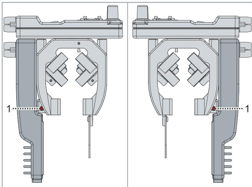
On both sides of the mover there is a set screw [1] for adjusting the position of the NCT electronics. The air gap between the NCT electronics and the module can be adjusted using the two set screws.
