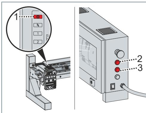
The *Power LED* [1] on the NCT electronics light up continuously.
