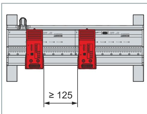
To initialize the movers, the distance between the movers must be at least 125 mm.
