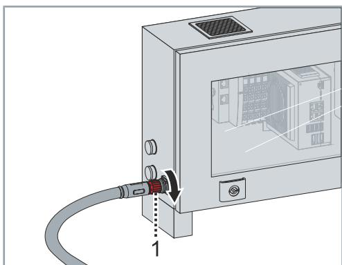
► Tighten the connector [1] with assembly tool [+]
