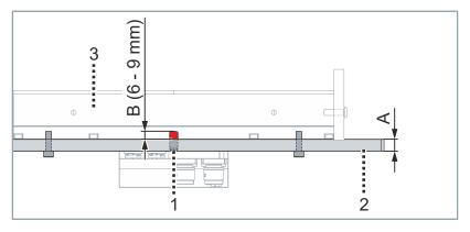
The length [C] of the D8 locating pins [1] for aligning the tile depends on the height [A] of the machine bed [3] and the projection [B] into the tile [3].
