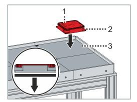
Position the mover [1] with transport securing device [2] directly on the tile [3]
