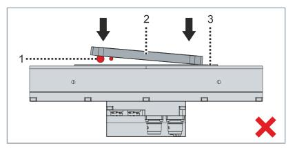
There must be no dirt or foreign objects [1] between the mover [2] and the cover [3] or the tile [4]. All dirt and foreign objects on the underside of the mover and on the surface of the cover or tile must be removed before force is applied to the mover.
