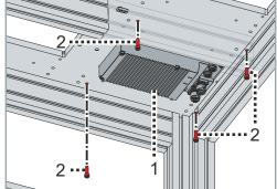
► Fasten the tile [1] with four screws [2]
