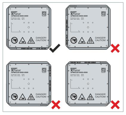
Make sure that you align the ID bumper correctly. The labels on the mover and on the ID bumper must have the same orientation. Incorrectly aligned ID bumpers can cause problems when controlling the movers.
