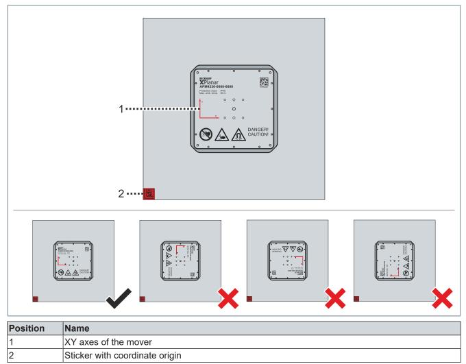
When placing the movers, make sure that the XY axes of the mover [1] correspond to the XY axes of the tile. The coordinate origin of the tile is used for orientation. Further information can be found in chapter "Tile orientation", [Page 62].
