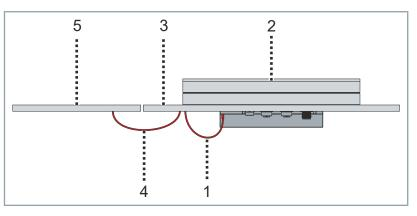
The functional conductor connection [1] of the tile [2] must be connected to the machine bed [3]. In addition, the machine bed [3] must be connected to another machine bed [5] with a functional conductor connection [4].
