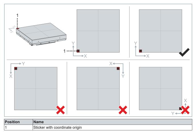
Make sure that all tiles have the same orientation. Use the coordinate origin [1] as a guide to align the tiles correctly.
