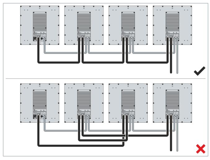
Only connect adjacent tiles with the power cable and the Ether-CAT G cable. Ideally, the power cable and the EtherCAT G cable of a tile are connected to the same other tile.
