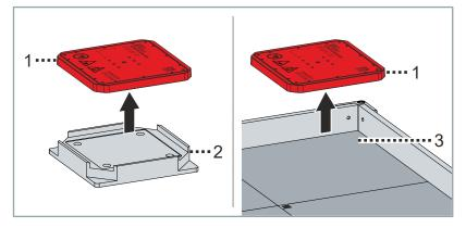
Remove the mover [1] from the transport securing device [2] and rotate it by 180°
