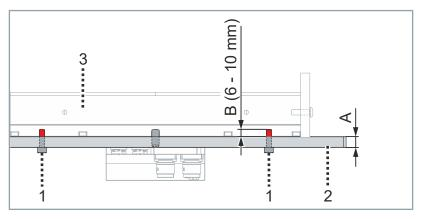
The length [C] of the M6 screws [1] for fastening the tile depends on the height [A] of the machine bed [2] and the screw depth [B] in the tile [3].
