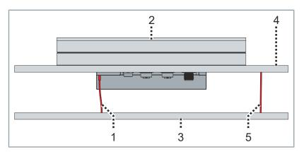
The functional conductor connection [1] of the tile [2] must be connected to the grounding bar [3]. In addition, the machine bed [4] must be connected to the grounding bar [3] with a functional conductor connection [5].
