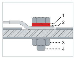
Ground the unpainted surface with spring washer [1], washer [2], nut [3] and bolt [4]
