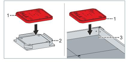
Place the mover [1] in the transport securing device [2] with the upper side facing upwards
