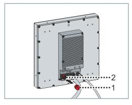
Insert and lock protective cap B17 [1] into the unused connection [2] of the tile
