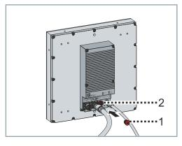
Insert protective cap M12 [1] into unused connection [2] of the tile
