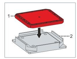
Place the mover [1] in the transport securing device [2] with the underside facing upwards
