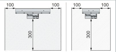
No magnetic materials may be used within a distance of 100 mm around a tile and 300 mm below a tile.
