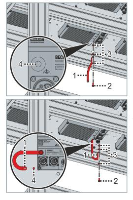
Screw the cable lug of the ground strap [1] to the machine bed [4] using a screw [2] and washers [3]
