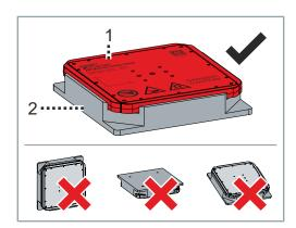
Transport the individual mover [1] with the safety pictograms facing upwards in the transport securing device [2] straight to the workplace or system
