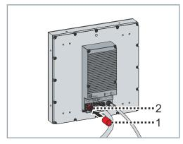
Insert the supplied protective cap B17 [1] into the unused connection [2] of the tile
