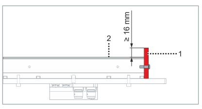
The mechanical protection [1] must protrude at least 16 mm beyond the stator surface [2].
