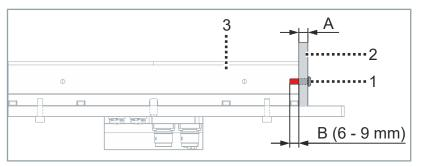
The length [C] of the M6 screws [1] for fastening the mechanical protection depends on the depth [A] of the safety equipment [2] and the screw depth [B] in the tile [3].
