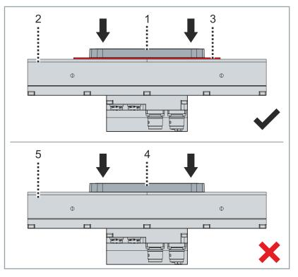
If you want to perform press-in processes on the mover, you must fit a cover [3] between the mover [1] and the tile [2].
