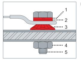
Ground the painted surface with spring washer [1], washer [2], contact washer [3], nut [4] and bolt [5]
