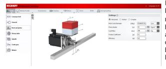
In the first step create the load case Conveyor belt. Microsoft Visual Studio and TC3 Motion Designer must be open. Furthermore, a <u>DC link [▶ 13]</u> must have been created, and an axis must have been added. Activate TC3 Motion Designer by doubleclicking on the created axis. Further information can be found in section: "Activating TC3 Motion Designer".
