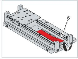
▶ Remove the protective cover [6] on the mounted magnetic plates onto which the machine slide is to be pushed. Do not dispose of the protective cover and keep it for subsequent transport of the machine or system.
