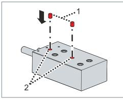
▶ Insert locating pins [1] into the holes of the coil unit [2]:
