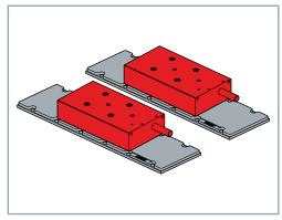
In a gantry structure, two parallel magnetic tracks each have a coil part. The coil parts are rigidly coupled and electrically connected in parallel. The movements are synchronized. Synchronization must be maintained at the best possible level even in the event of a drive error.
