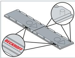
▶ Place the magnetic plate [4] on the locating pins [3]
