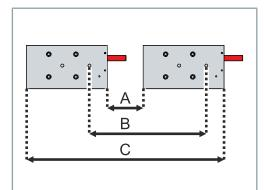
This illustration shows an example of an arrangement of two coil parts with cables in the same direction.
