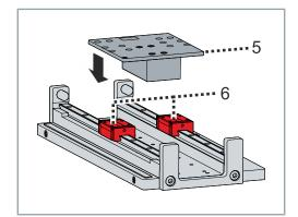
▶ Place the assembled coil unit including the machine carriage [5] on the guide carriage [6]
