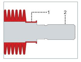
► Pull the front end of the bellows [1] over the spindle extension [2] and bring it into position
