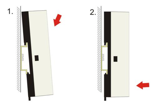
To release the CU8871-0000 from the mounting rail:
