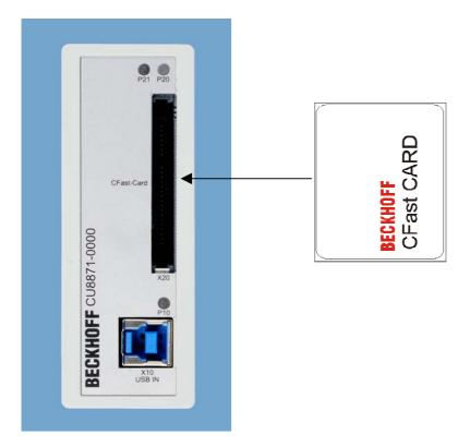
As soon as the card is inserted, the LED (P20) lights up green. The red LED (P21) flashes up shortly, too.
