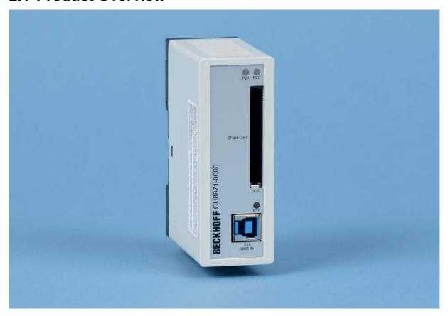
The CU8871-0000 offers a CFast socket with USB connector in a compact housing for DIN rail mounting. CFast Flash cards are used in the industrial environment as data memory for process and control data. The CFast cards are hot-plug capable in the CU8871 and can hence be plugged and unplugged like removable data storage devices for exchanging data with other PCs during operation.
