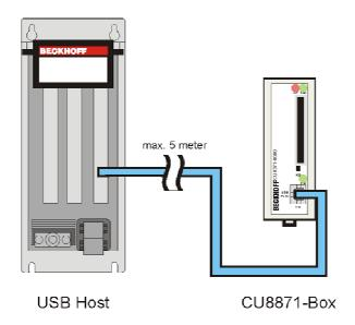
The CFast card adapter is connected to a USB host via a standard USB cable. The maximum length for the wire is 3 meters. For correct operation, use USB 3.0 suitable wire.
