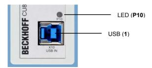
The USB-CFast card adapter does not need any additional power supply. The power supply (5V DC) is realized by the USB connector (1). The LED **P10** lights green when power supply is connected.
