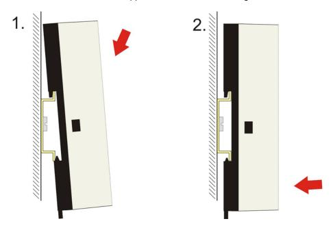
To release the CU8870-0000 from the mounting rail
