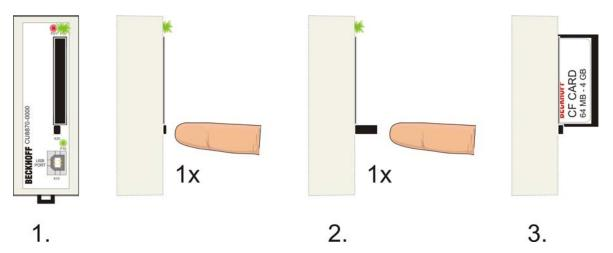
For ejecting the CF card press the small button below the CF slot. By pressing the button once the button expands. Pressing the button the second time the CF card ejects. The button engages again. The green LED (P20) extinguishes.
