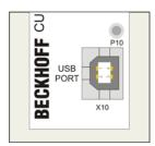
The CF card reader does not need any additional power supply. The power supply (5 V DC) is realized by the USB connector. The LED P10 lights green when power supply is connected.
