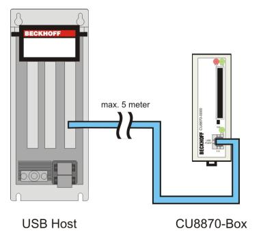
The CF card reader is connected to a USB host via a standard USB cable. The maximum length for the wire is 5 meters. For correct operation, use USB 2.0 suitable wire.
