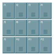
The meaning of the function keys, *F1* to *F10*, is determined by the software and is displayed at the bottom edge of the display.
