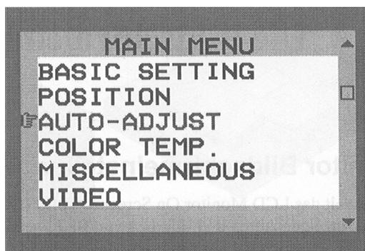
The control functions are divided into seven categories that are displayed in the main menu. Scroll through the menu options by repeatedly pressing the "Function up" and "Function down" buttons. By pressing the "Adjustment up" and "Adjustment down" keys you reach the sub-menus in each function group. Each menu item is described below.
