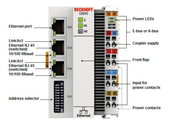
The CX8090 is a control system with a switched Ethernet port. It supports protocols such as real-time Ethernet, ADS UDP/TCP, Modbus TCP client/server or open TCP/IP-UDP/IP communication. K-Bus or E-Bus terminals can be attached as required; the CX8090 automatically recognizes the type of I/O system connected during the start-up phase. The control system is programmed with TwinCAT via the fieldbus interface or the additional Ethernet interface.
