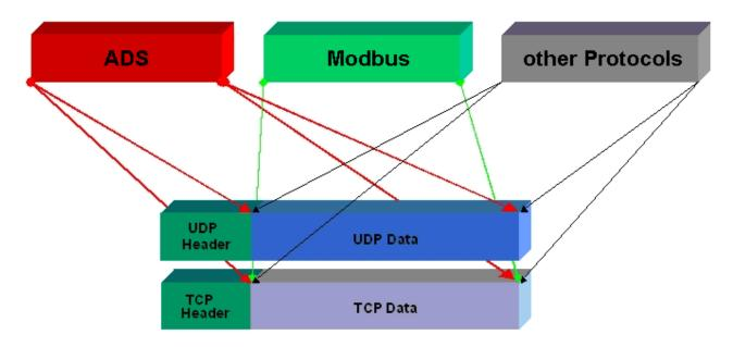
ADS can be used on top of either TCP or UDP, but ModbusTCP is always based on TCP/IP.
