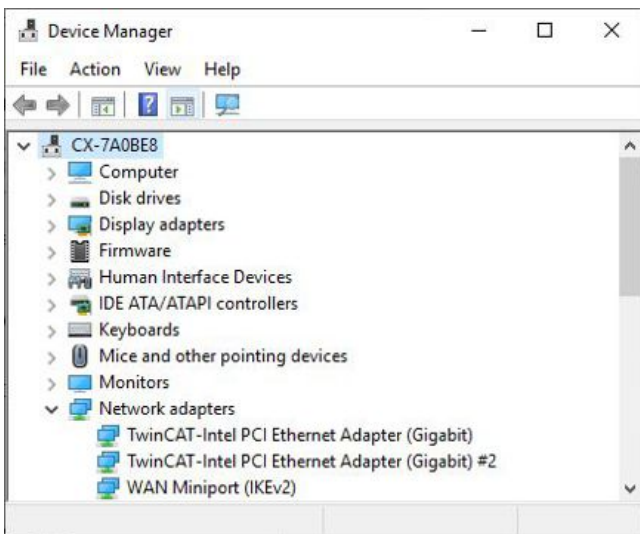
Fig. 30: Windows 10, identification of the Ethernet interfaces (X000, X001) in the device manager.
