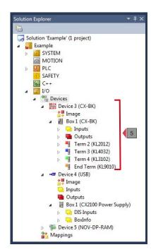
Fig. 32: CX20x0 Embedded PC in the tree view of TwinCAT 3, with attached EtherCAT Terminals (left) or Bus Terminals (right).
