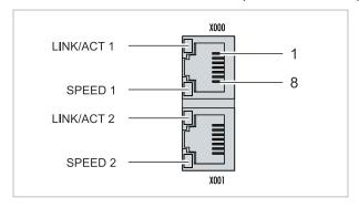
Fig. 7: Ethernet interfaces X000, X001.
