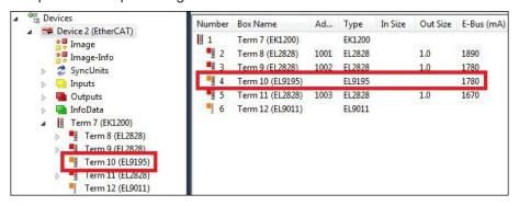
Fig. 22: Identifying a passive EtherCAT Terminal in TwinCAT.
