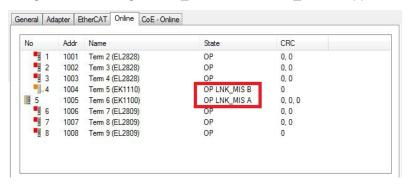
Although the connection between the Bus Couplers is interrupted, the EtherCAT Terminals connected to the EK1100 Bus Coupler show no fault.
