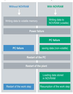
Fig. 34: Controller behavior with and without NOVRAM.
