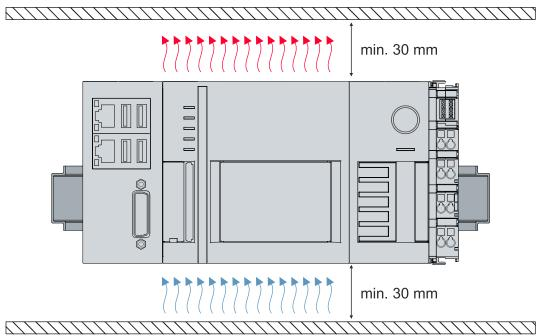
Fig. 21: Embedded PC CX20x0, horizontal installation position.
