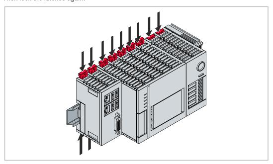
⇒ You have installed the Embedded PC successfully. Double-check the correct installation and latching of the Embedded PC on the mounting rail.
