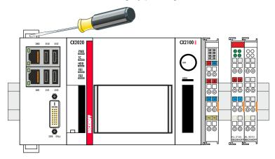
2. Pull the orange strap on the power supply unit and gently remove the device from the DIN rail.
