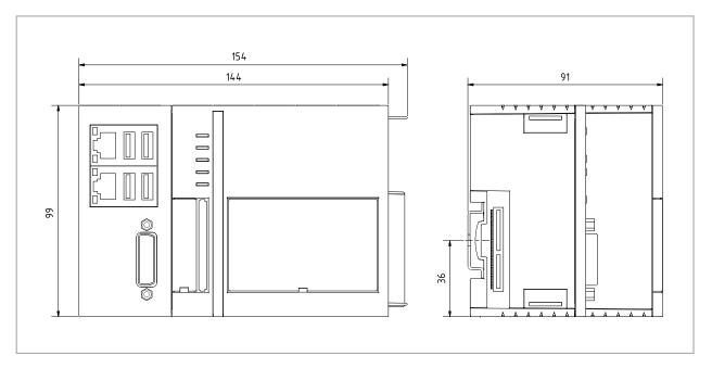
Fig. 20: CX2040 Embedded PC, dimensions.
