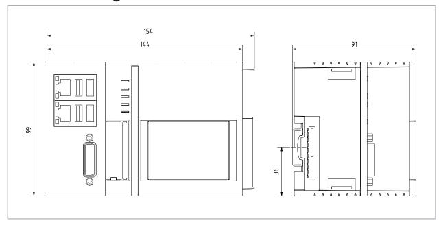
Fig. 19: CX2020 and CX2030 Embedded PC, dimensions.
