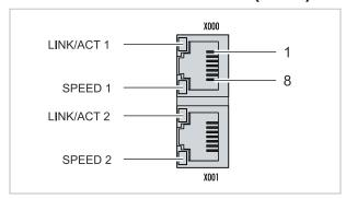
Fig. 17: PROFINET RT interface X300.
