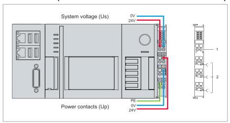
Fig. 24: Connections for system voltage (Us) and power contacts (Up).
