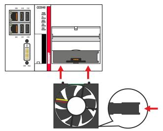
⇒ Close the front flap. You have successfully changed the fan cartridge if the fan starts up again.
