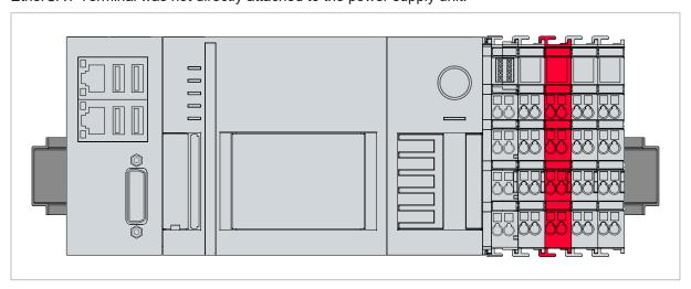
Fig. 23: Passive EtherCAT Terminals, permissible installation.
