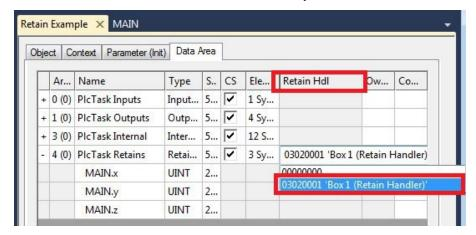
After selecting a Retain Handler as a target, the symbols in the tree view are linked and a mapping is created.
