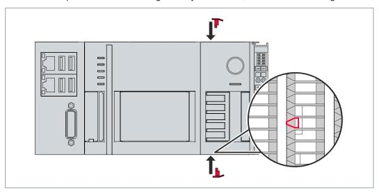
⇒ The bar clips have been installed successfully, if they don't protrude and are level with the cooling fins of your modules.
