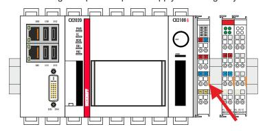
3. Lift the bar clips with the aid of a screwdriver and remove the bar clips.
