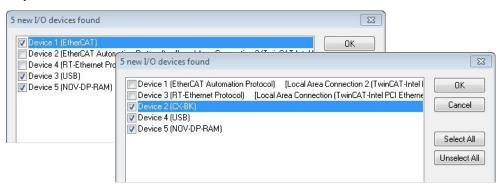
For Embedded PCs with connected Bus Terminals (K-bus) a Bus Coupler device (CX-BK) is displayed. For EtherCAT Terminals (E-bus) the EtherCAT coupler is added automatically.
