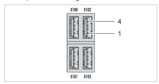
Fig. 6: USB interfaces (X100, X101, X102, X103).
