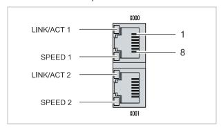
Fig. 14: EtherCAT slave interface X300.
