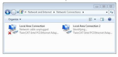
Fig. 28: Windows 7, Identification of the Ethernet interfaces (X000, X001) in the Network and Sharing Center.
