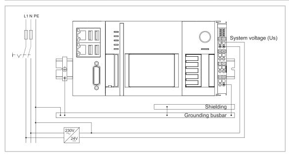
Fig. 25: Connection example with a CX20x0.
