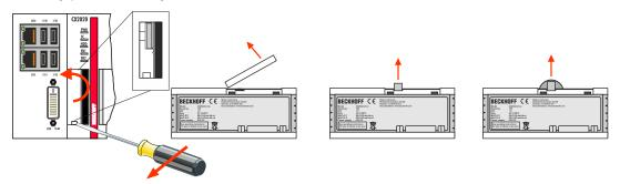
3. Push the new battery into the battery compartment. The positive pole points to the left towards the DVI-l interface.
