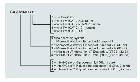
Fig. 4: Nomenclature for the basic CPU module.
