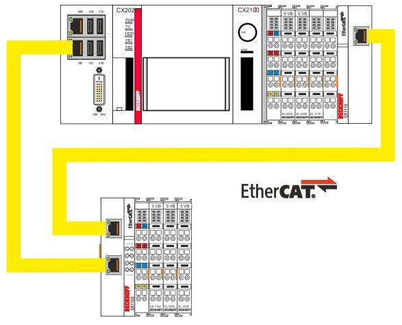
Fig. 33: Smallest possible configuration for EtherCAT cable redundancy.
