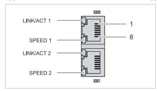
Fig. 13: EtherCAT master interface X300.
