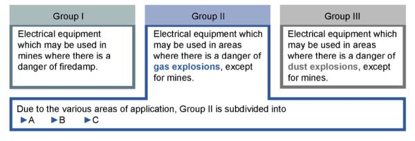
This subdivision is graded in accordance with the properties of the explosive atmosphere in which the equipment is used and is based on the minimum ignition current ratio of representative gases.
