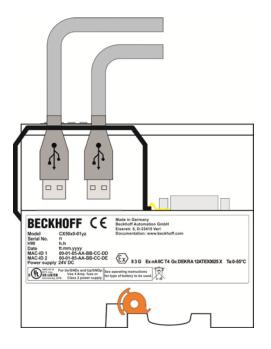
2. When the USB plugs are placed the cables must be fixed with cable straps to the bracket.
