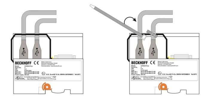
3. The tensile strength of the wire must be checked and if necessary the cable straps must be retightened. The remains of the straps can be cut off with nippers or a side cutter.
