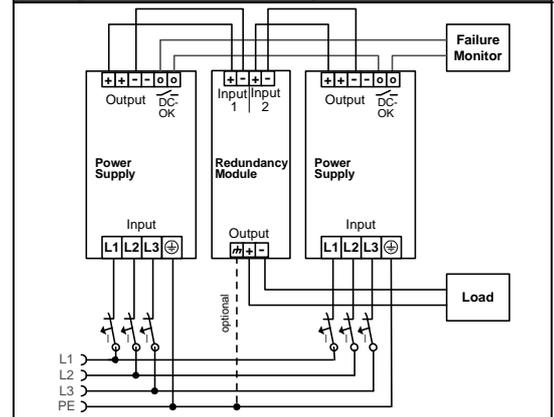
**Wiring scheme - n+1 redundancy**
