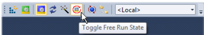
Fig. 92: TwinCAT can also be switched to this state by using a button (TwinCAT 3)
