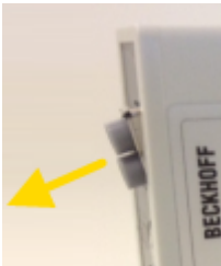
Fig. 24: Slanting installation of the optical fiber socket
