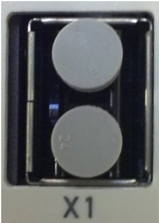
Fig. 34: Blind plugs in unused sockets
