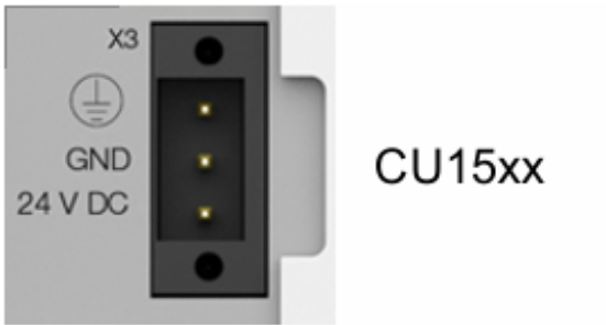
Fig. 15: Pin assignment of the connection terminal (X3)
