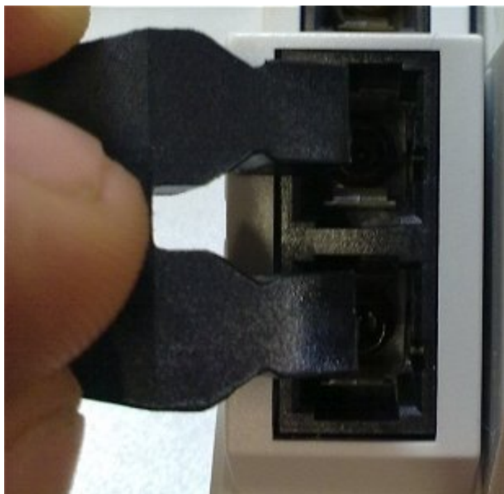
Fig. 31: Blind plugs in unused sockets
