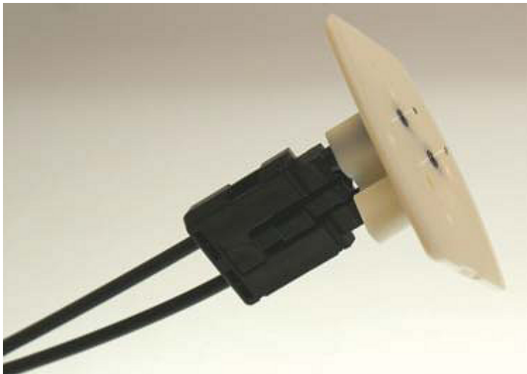
Fig. 38: Sanding gauge with protruding fiber ends
