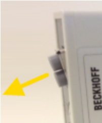
Fig. 24: Slanting installation of the optical fiber socket
