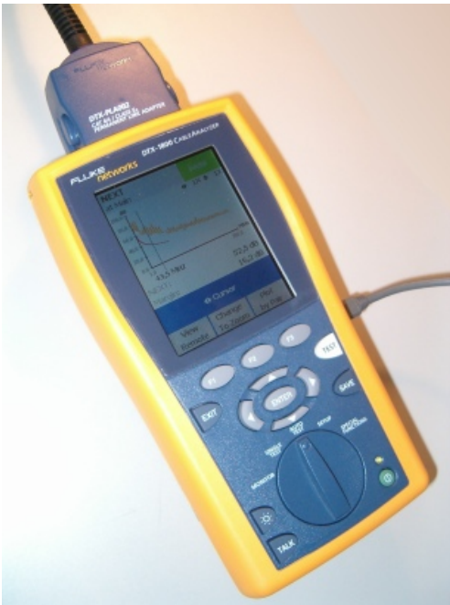
Fig. 34: Example illustration of a cable certifier
