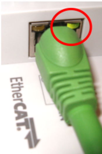
Fig. 33: Link LED on Ethernet devices
