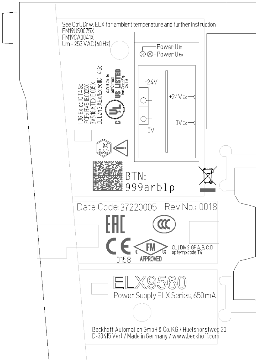
Fig. 2: ELX9560 with date code 37220005, BTN 999arb1p and marking für ATEX, IECEX and cFMus
