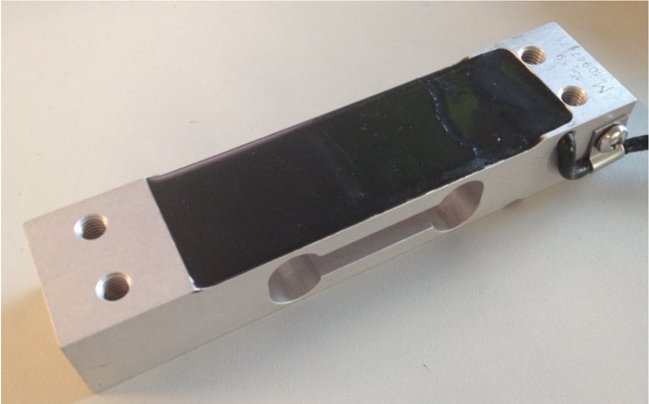
Fig. 37: Example of a load cell
