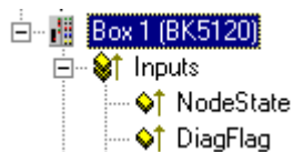
Fig. 142: TwinCAT tree: Diagnostic Inputs
