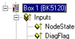
Fig. 139: Diagnosis of inputs in the TwinCAT tree
