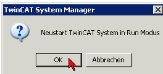
Fig. 157: Restarting TwinCAT in RUN mode
