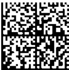
Fig. 3: Example DMC 1P072222SBTNk4p562d71KEL1809 Q1 51S678294
