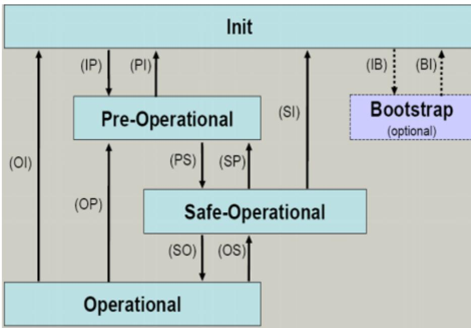
Fig. 31: States of the EtherCAT State Machine
