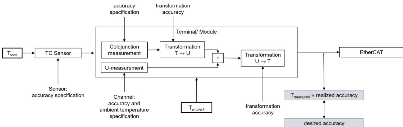
The given voltage specification is decisive for the achievable temperature measuring accuracy. It is applied to the possible thermocouple types in the following.
