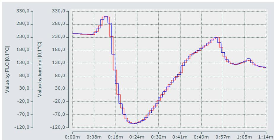
Fig. 192: Blue: temperature values from the PLC calculation; red: PDO values in the temperature measurement range
