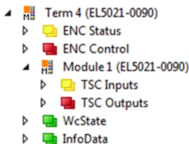
Fig. 159: TwinSAFE SC component process data, example EL5021-0090
