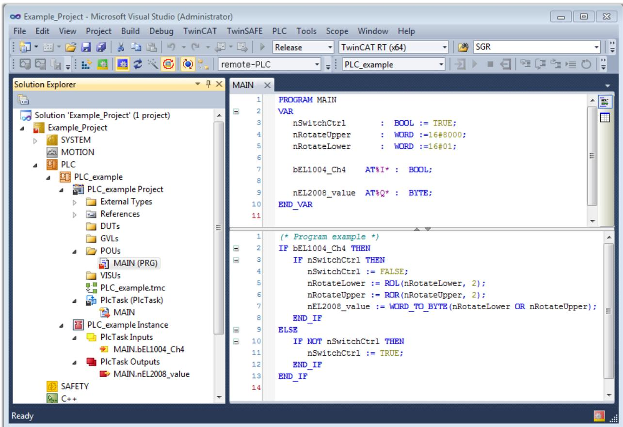
Fig. 81: Sample program with variables after a compile process (without variable integration)
