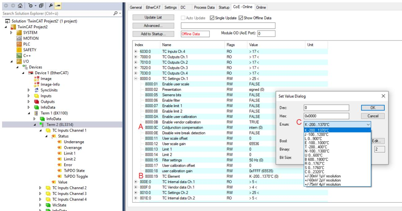
Fig. 170: Setting the measuring range
