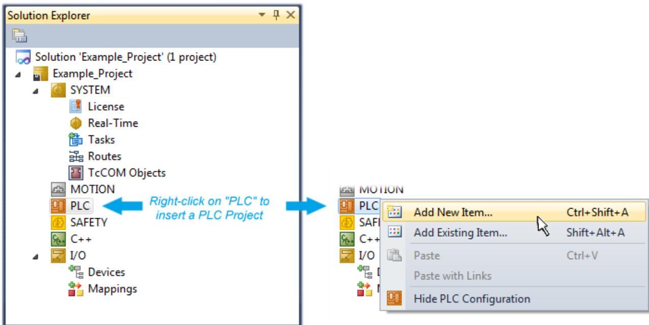
Fig. 78: Adding the programming environment in “PLC”
