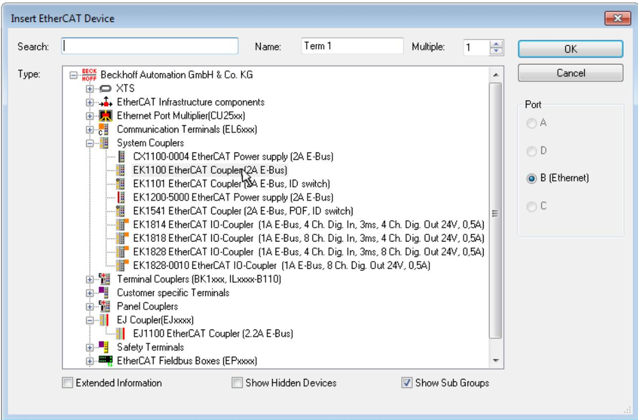
Fig. 113: Selection dialog for new EtherCAT device
