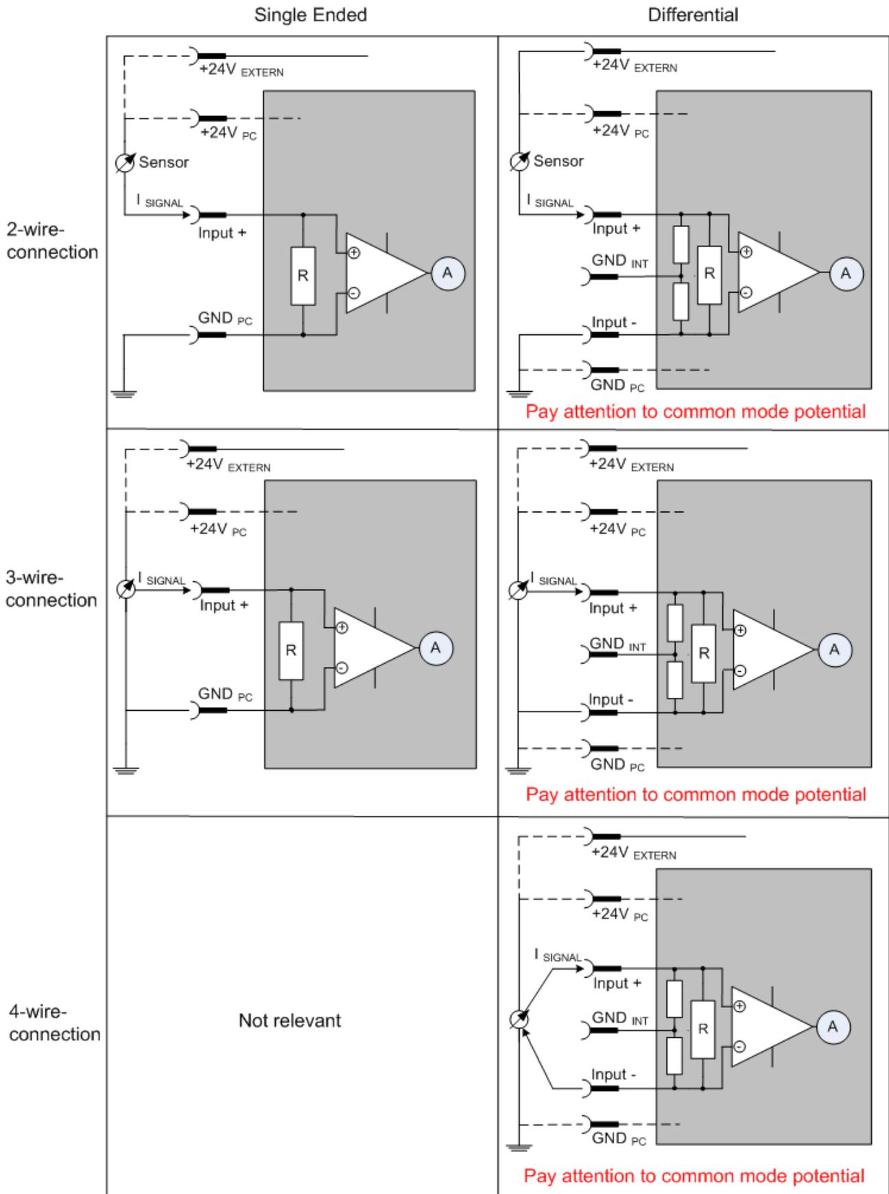
Fig. 186: 2-, 3- and 4-wire connection at single-ended and differential inputs
