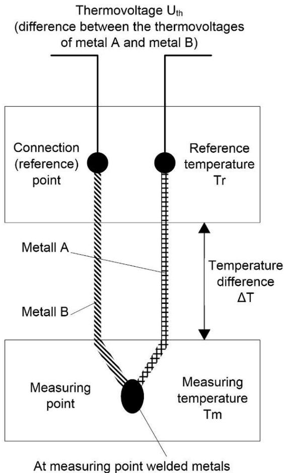
Fig. 23: Structure and principle of a thermocouple
