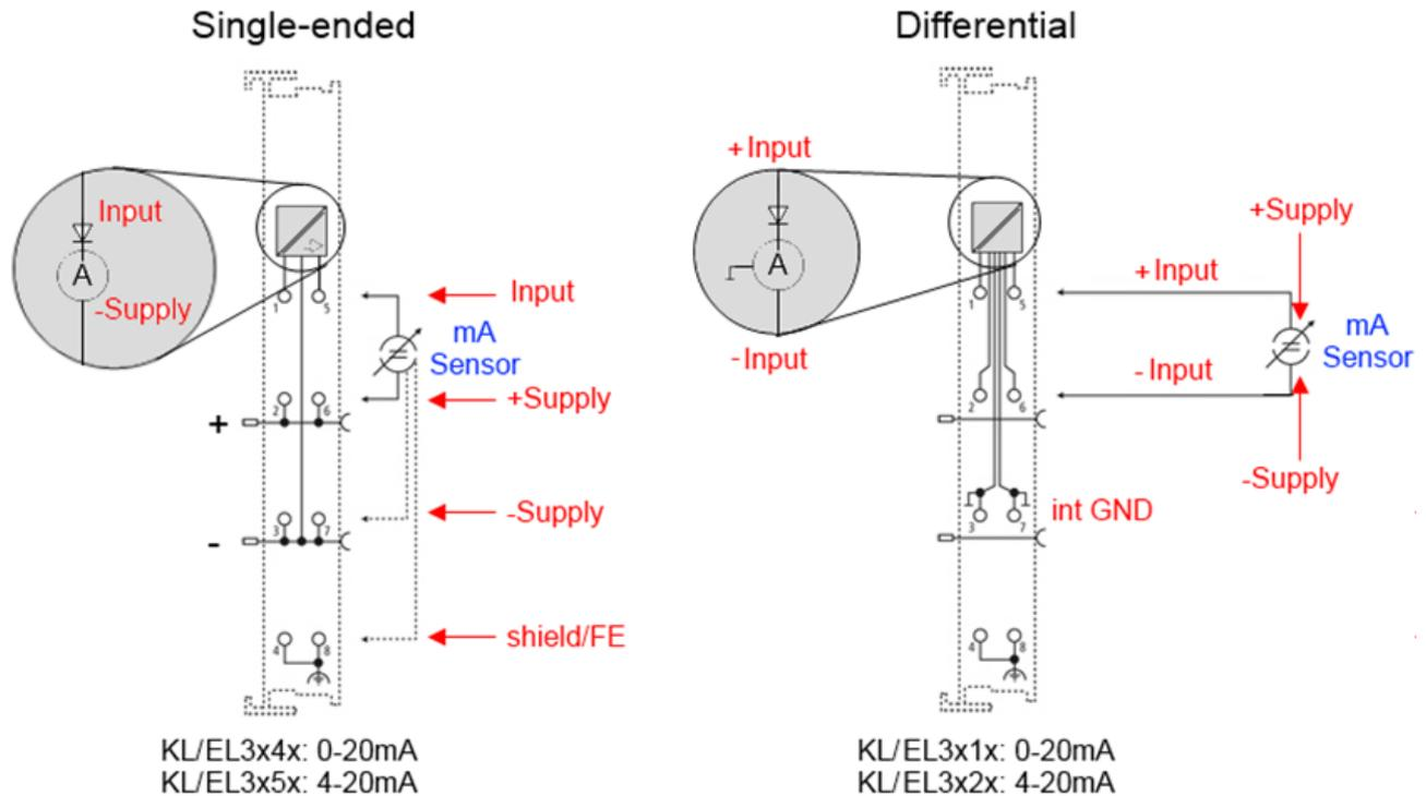
Fig. 185: Connection of externally supplied sensors
