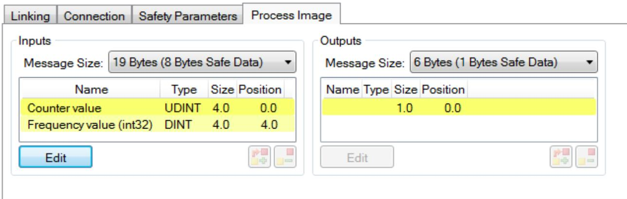
Fig. 163: Selecting the process data size and the process data
