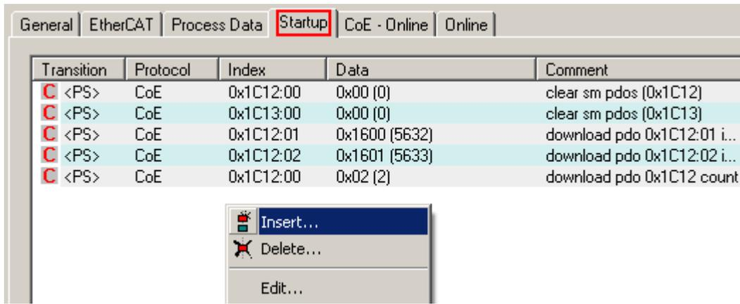
Fig. 33: Startup list in the TwinCAT System Manager
