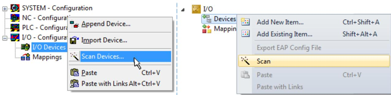
Fig. 119: Scan Devices (left: TwinCAT 2; right: TwinCAT 3)
