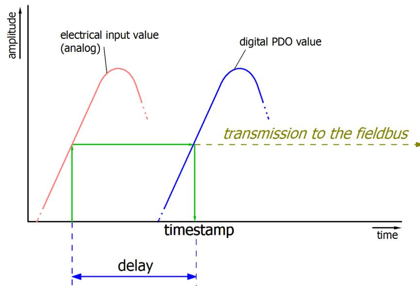
Fig. 191: Diagram signal delay (linear)
