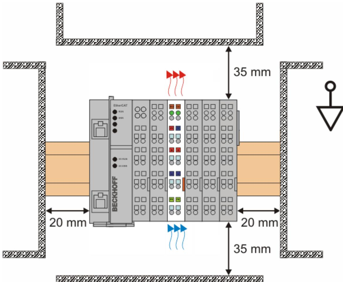
Fig. 49: Recommended distances for standard installation position
