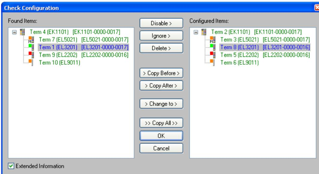
Fig. 181: Typical result after scanning an EtherCAT system
