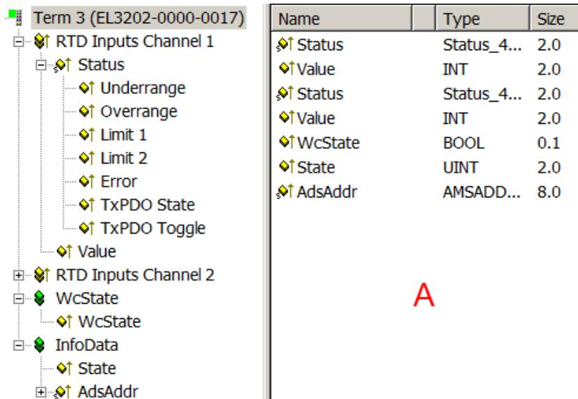
Fig. 177: EL32xx-0000-0017 process image in the TwinCAT 2.11 representation
