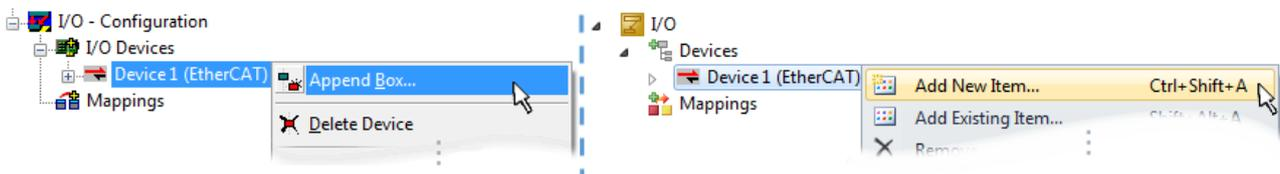
Fig. 112: Appending EtherCAT devices (left: TwinCAT 2; right: TwinCAT 3)
