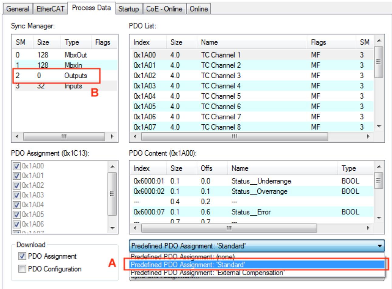
Fig. 167: TwinCAT System Manager with predefined PDO option "Standard"
