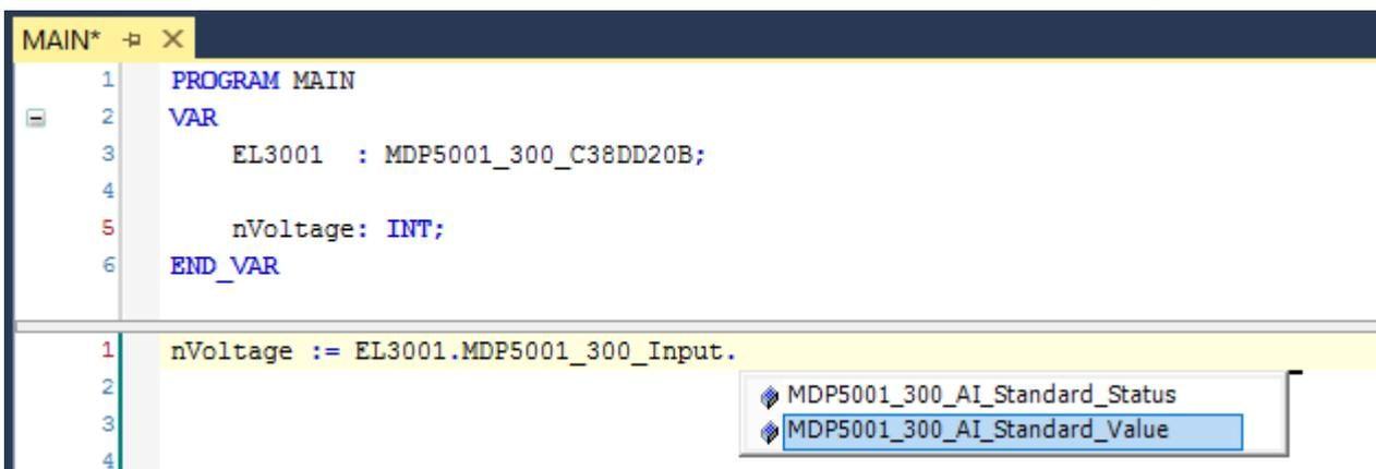
Fig. 90: Reading a variable from the structure of the process data
