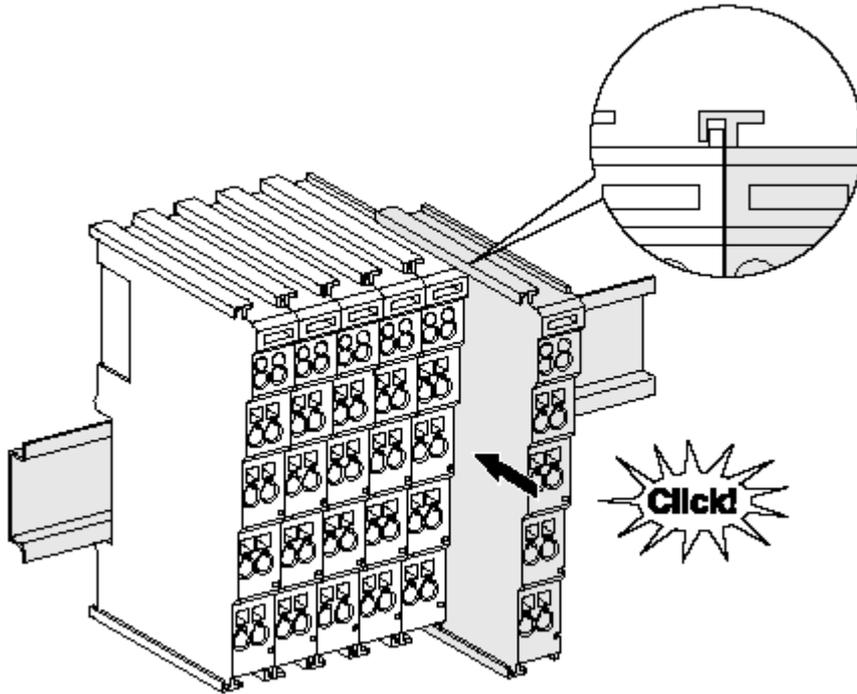
Fig. 37: Attaching on mounting rail
