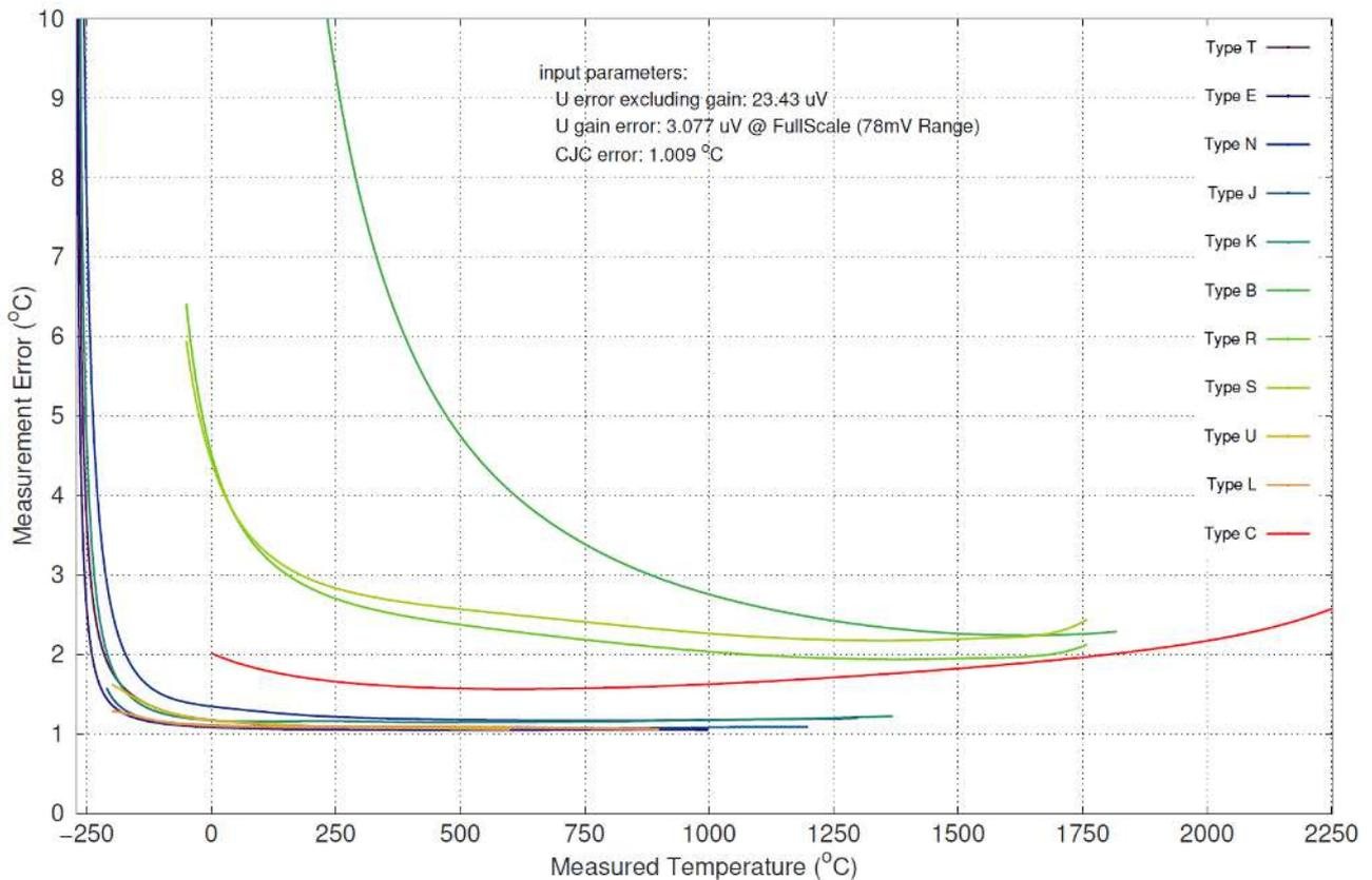
Fig. 26: Example of a thermocouple evaluation uncertainty analysis with an EL331x thermocouple terminal
