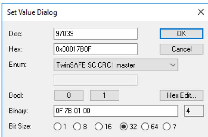
Fig. 166: Entering the safety address and the CRC
