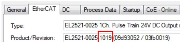
Fig. 124: Detection of EtherCAT terminal with revision -1019
