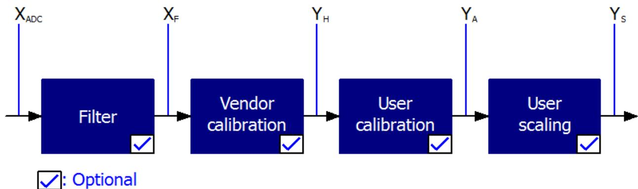
Fig. 171: Calculation of process data
