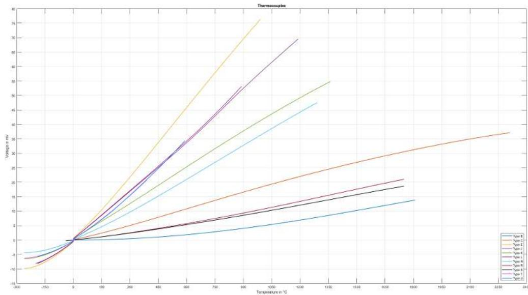
Fig. 24: Characteristic voltage/temperature curves of different thermocouple types
