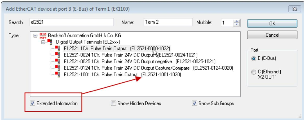
Fig. 114: Display of device revision
