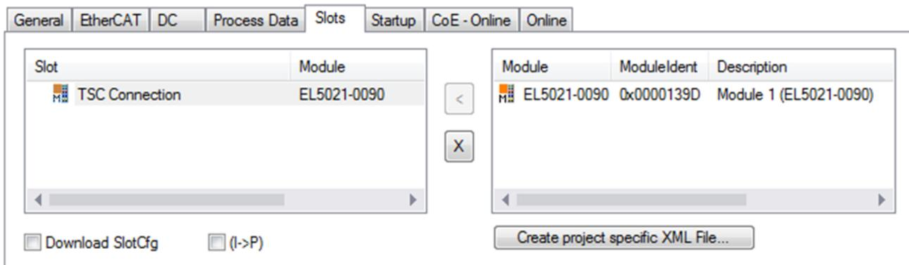
Fig. 158: Adding the TwinSAFE SC process data under the component, e.g. EL5021-0090
