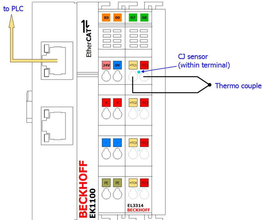
Fig. 193: Structure of the sample program for "separate temperature calculation with CJC in the PLC"
