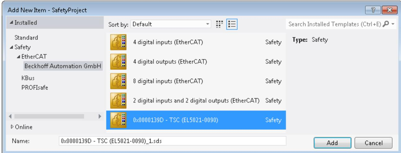
Fig. 160: Adding a TwinSAFE SC connection
