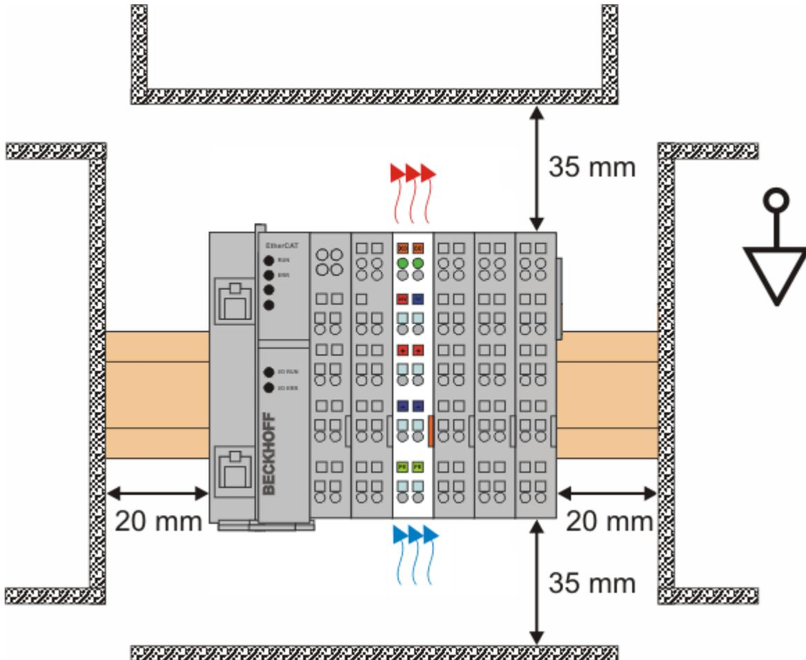
Fig. 47: Recommended distances for standard installation position
