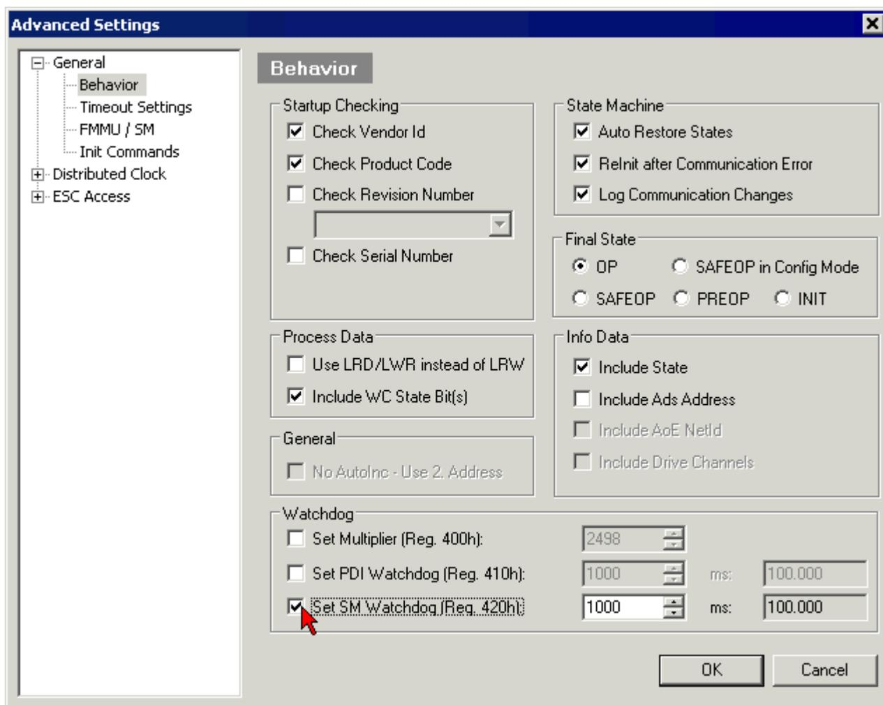
Fig. 30: EtherCAT tab -> Advanced Settings -> Behavior -> Watchdog
