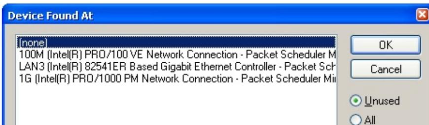
Fig. 110: Selecting the Ethernet port
