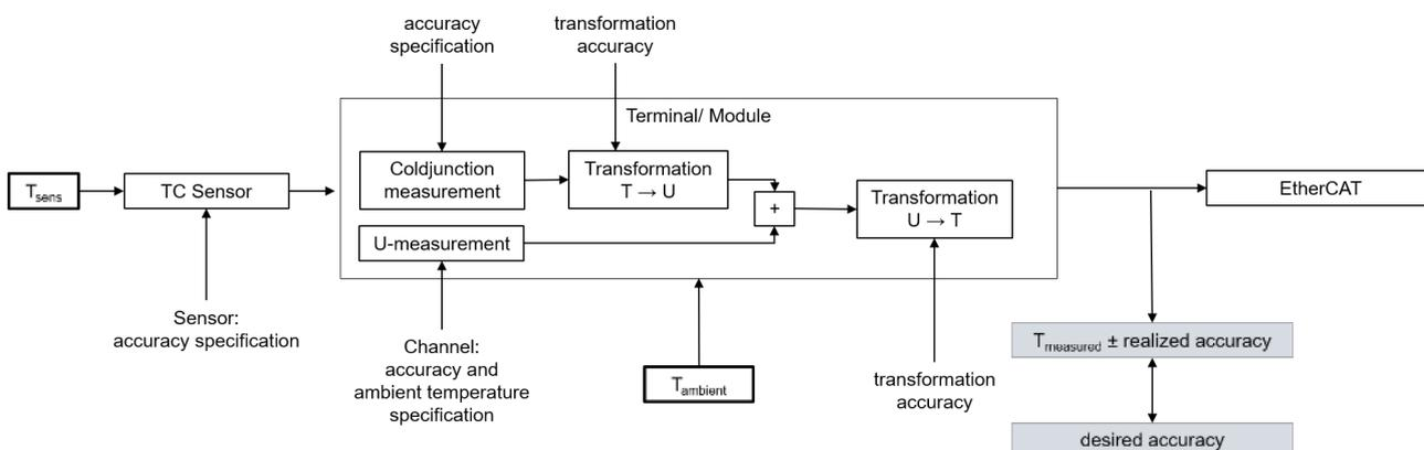
Fig. 25: Concatenation of the uncertainties in temperature measurement with thermocouples
