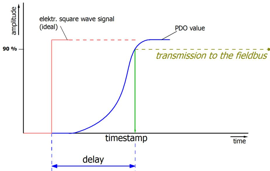
Fig. 190: Diagram signal delay (step response)
