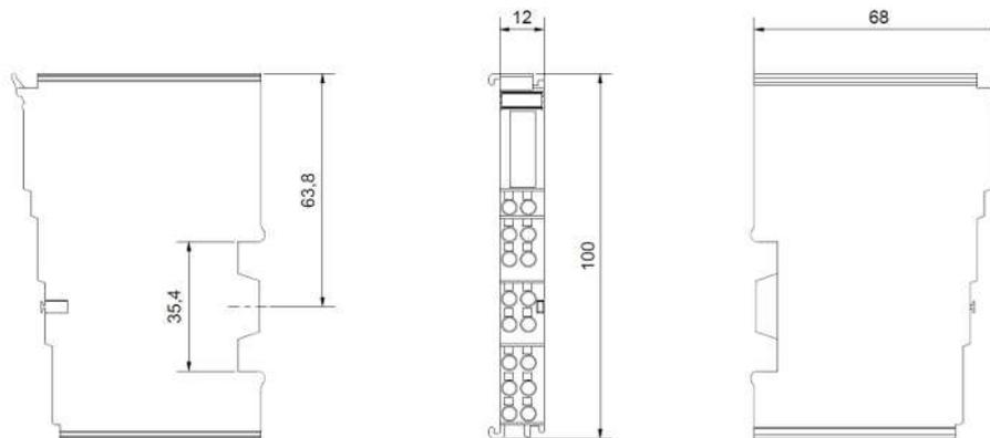
Fig. 21: Technical drawing | housing EL-12-16 pin
