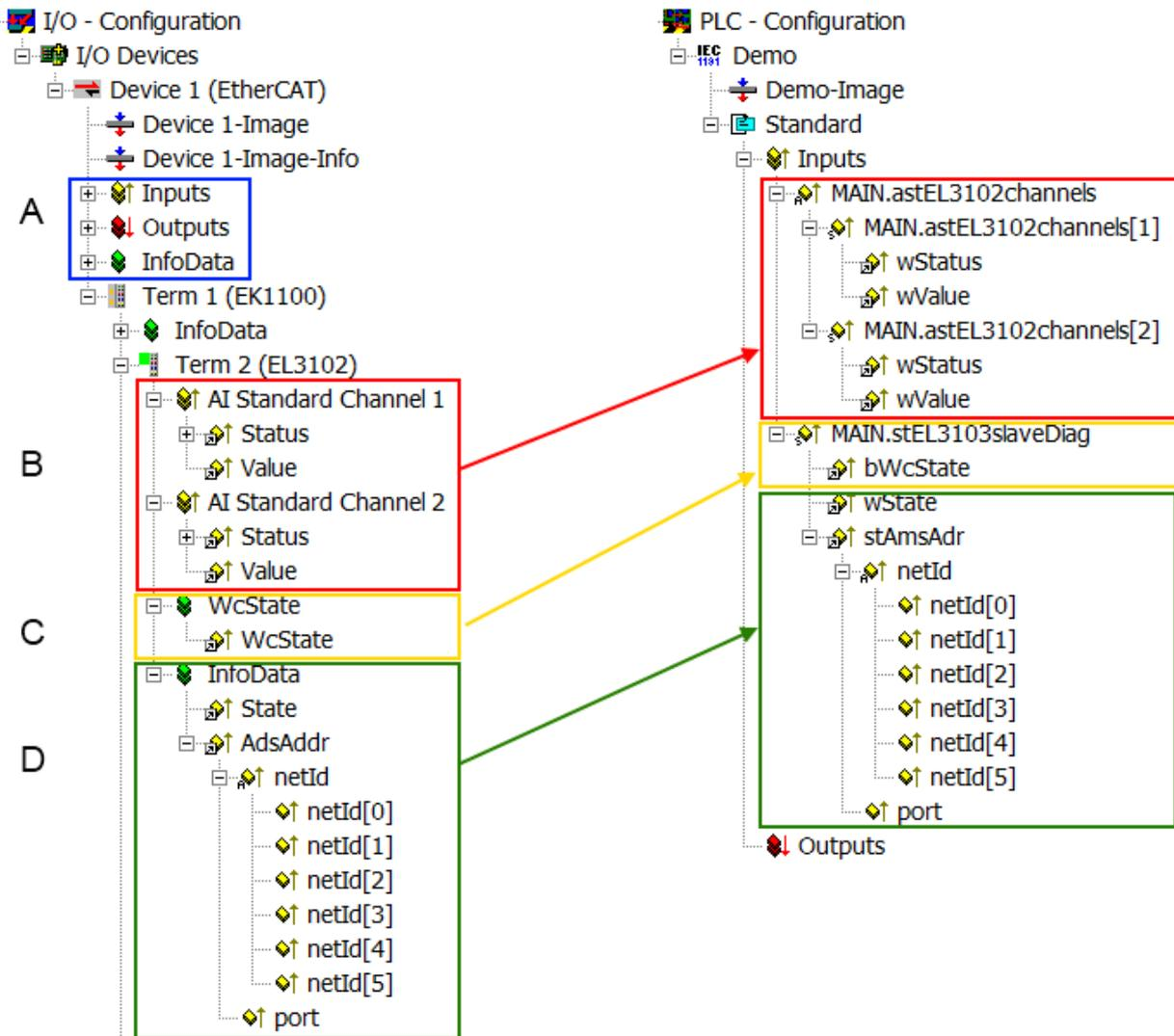
Fig. 150: Basic EtherCAT Slave Diagnosis in the PLC
