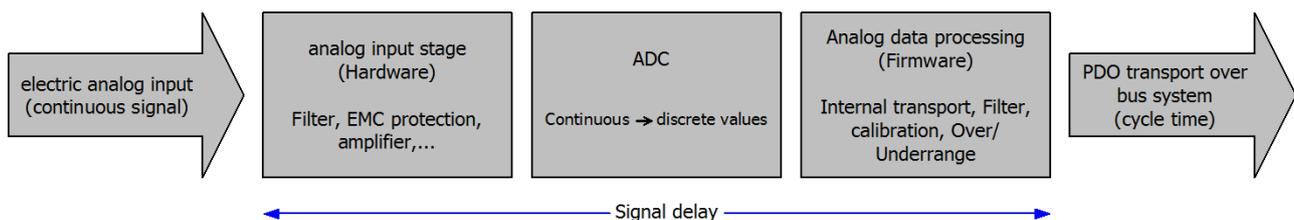
Fig. 189: Signal processing analog input
