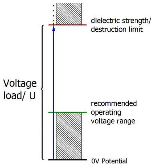
Fig. 188: Recommended operating voltage range
