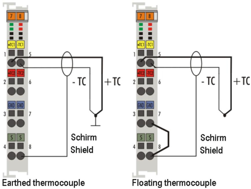
Fig. 44: Connection methods for earthed and earth-free thermocouples
