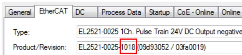
Fig. 123: Installing EtherCAT terminal with revision -1018
