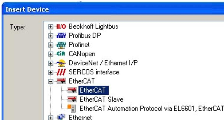
Fig. 109: Selecting the EtherCAT connection (TwinCAT 2.11, TwinCAT 3)
