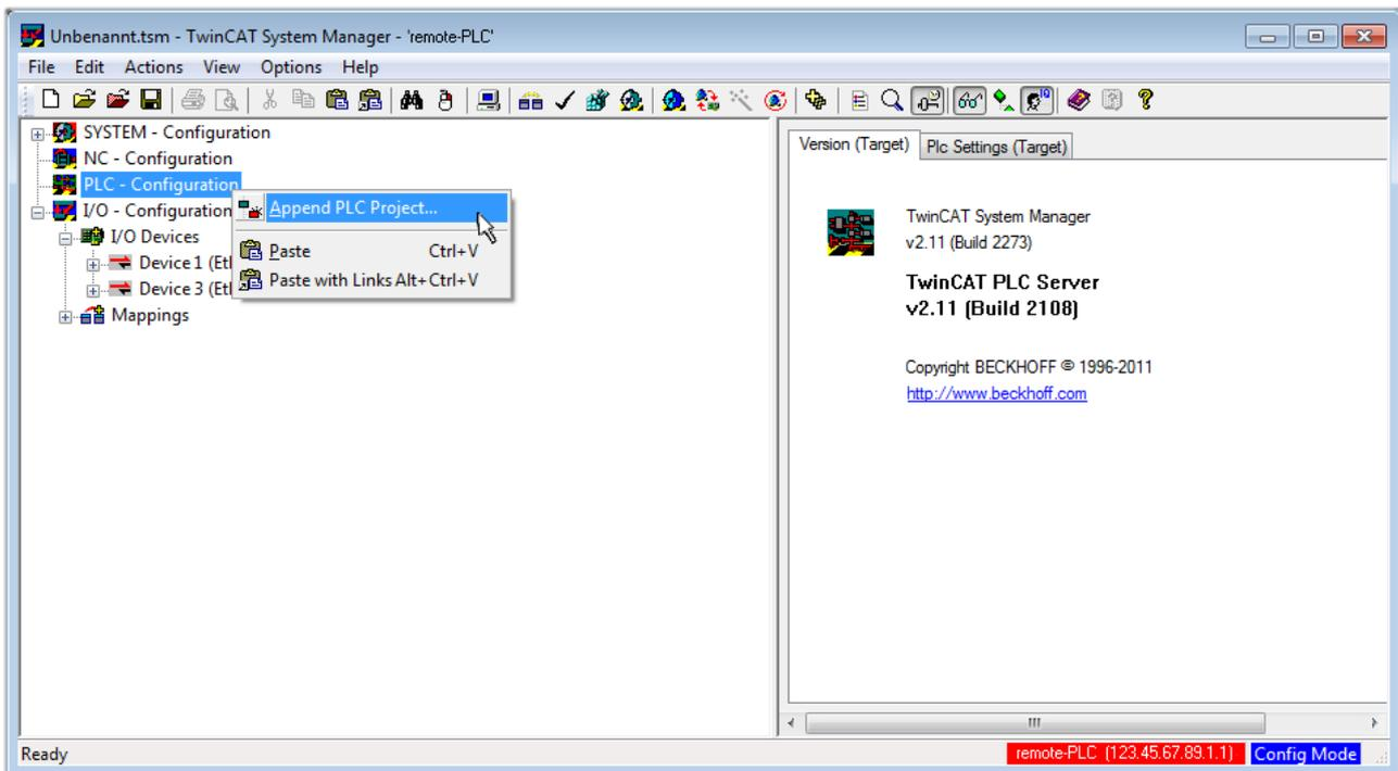
Fig. 61: Appending the TwinCAT PLC Control project
