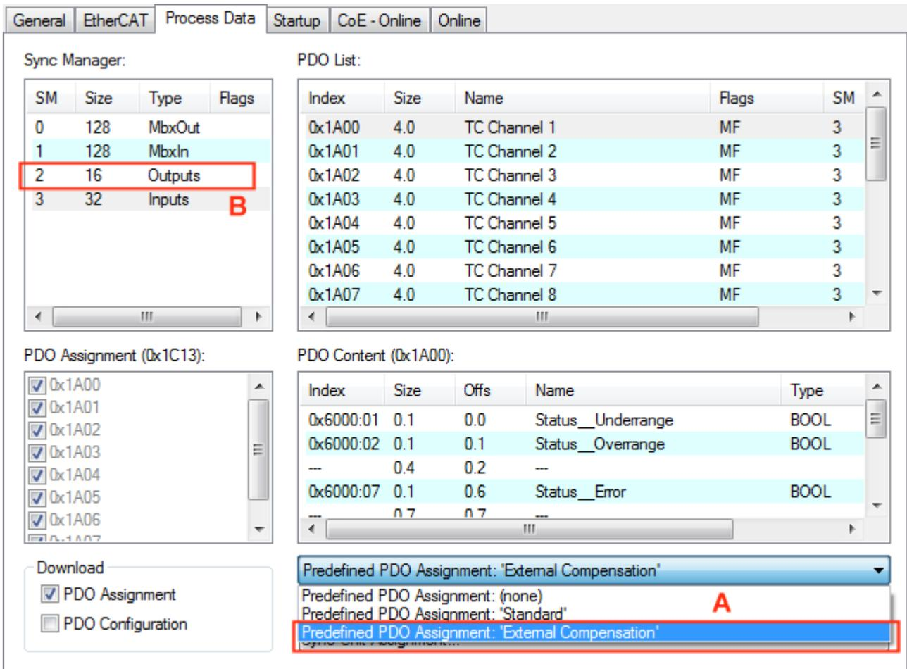
Fig. 168: TwinCAT System Manager with the predefined PDO selection "External Compensation"
