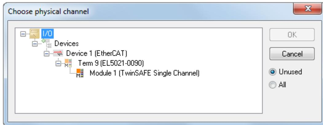
Fig. 161: Creating a link to TwinSAFE SC terminal
