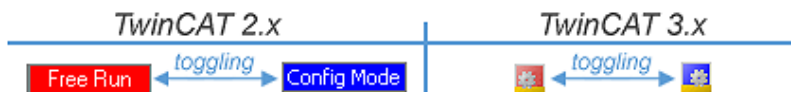
Fig. 107: Displaying of “Free Run” and “Config Mode” toggling right below in the status bar
