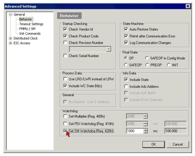
Fig. 30: eEtherCAT tab -> Advanced Settings -> Behavior -> Watchdog
