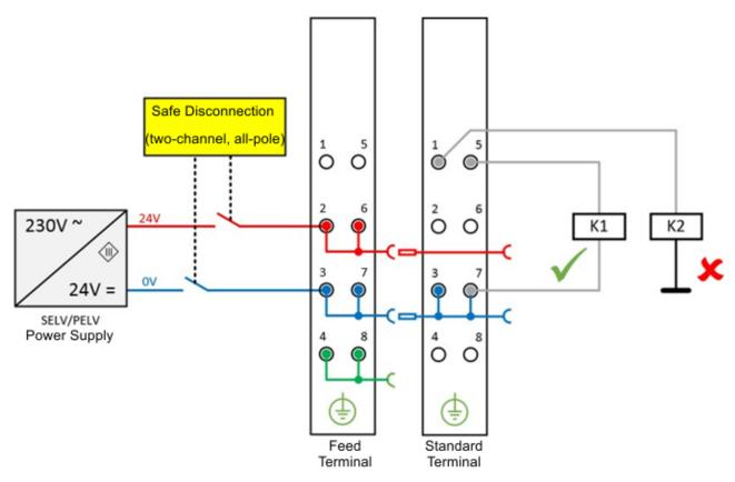
Fig. 5: Ground connection of the load: correct (K1) and incorrect (K2)
