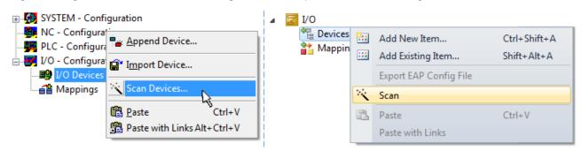
Fig. 118: Scan Devices (left: TwinCAT 2; right: TwinCAT 3)
