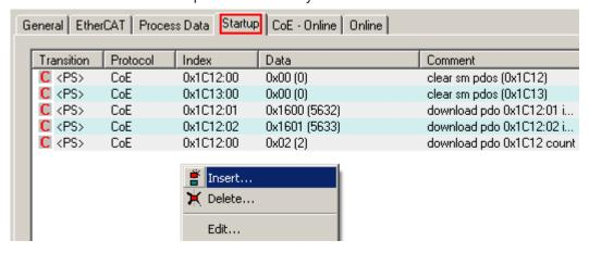
Fig. 33: Startup list in the TwinCAT System Manager
