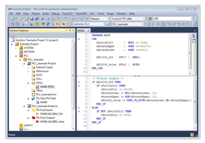
Fig. 79: Example program with variables after a compile process (without variable integration)
