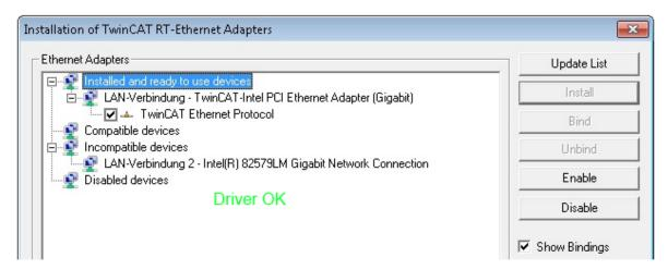
Fig. 96: Exemplary correct driver setting for the Ethernet port
