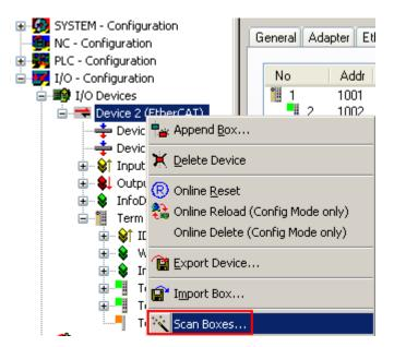
Fig. 158: Scan the subordinate field by right-clicking on the EtherCAT device
