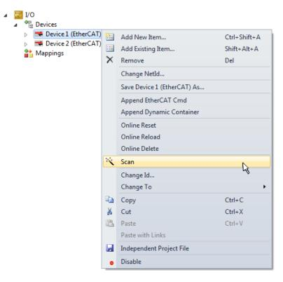
Fig. 75: Reading of individual terminals connected to a device
