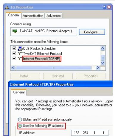
Fig. 98: TCP/IP setting for the Ethernet port
