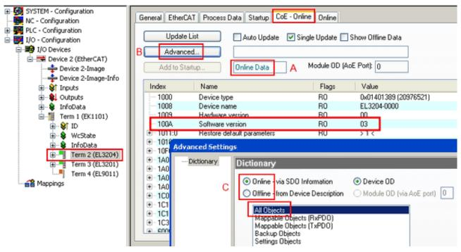
Fig. 163: Display of EL3204 firmware version
