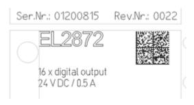
Fig. 1: EL2872 with revision 0022 and serial number 01200815
