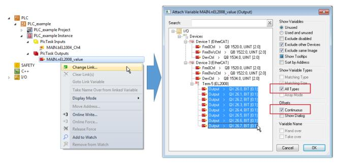
Fig. 83: Selecting several PDOs simultaneously: activate "Continuous" and "All types"
