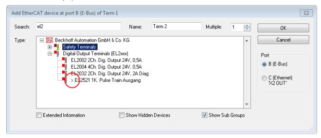
Fig. 103: Indication of an online recorded ESI of EL2521 as an example
