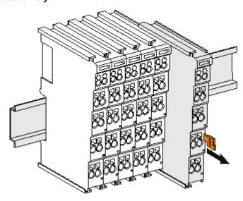
Fig. 38: Disassembling of terminal
