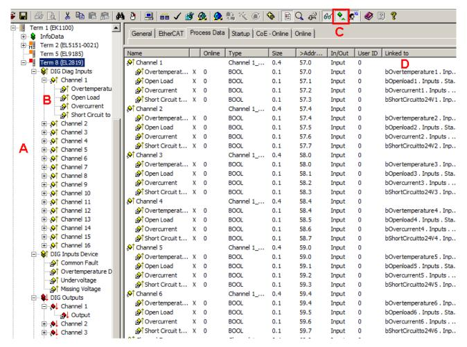
Fig. 19: EL2819 Online illustration of the process data and structural contents in the System Manager
