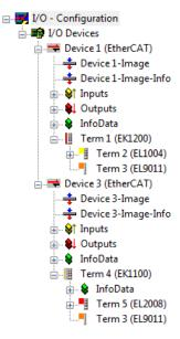
Fig. 55: Mapping of the configuration in the TwinCAT 2 System Manager
