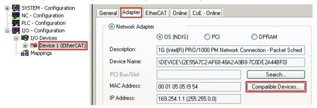
Fig. 94: EtherCAT device properties (TwinCAT 2): click on "Compatible Devices..." of tab "Adapter"
