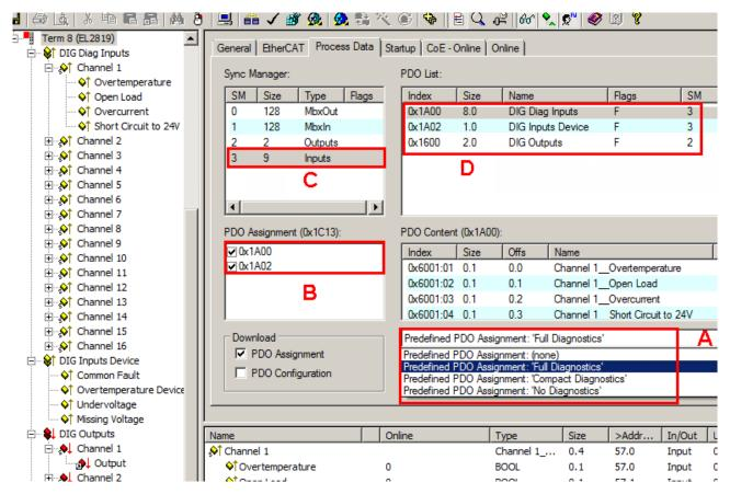
Fig. 20: EL2819 "Process Data" tab
