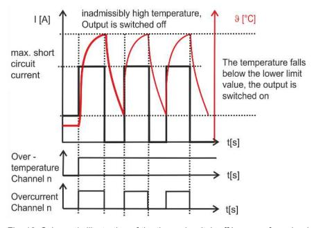
Fig. 16: Schematic illustration of the thermal switch-off in case of overload
