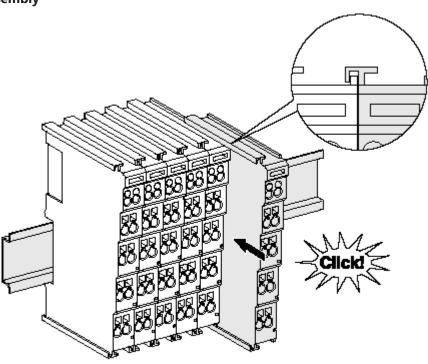
Fig. 37: Attaching on mounting rail
