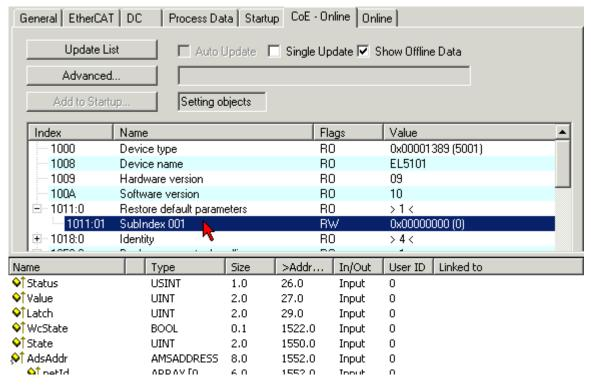
Fig. 169: Selecting the Restore default parameters PDO
