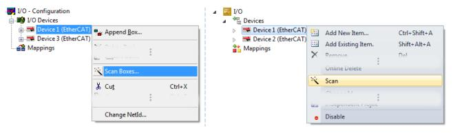
Fig. 125: Manual triggering of a device scan on a specified EtherCAT device (left: TwinCAT 2; right: TwinCAT 3)
