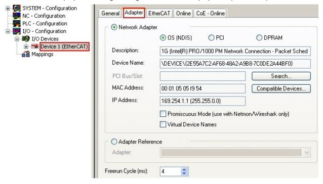
Fig. 110: EtherCAT device properties (TwinCAT 2)
