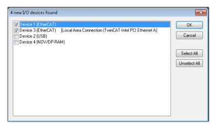
Fig. 73: Automatic detection of I/O devices: selection of the devices to be integrated
