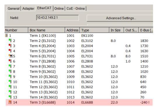
Fig. 155: Illegally exceeding the E-Bus current
