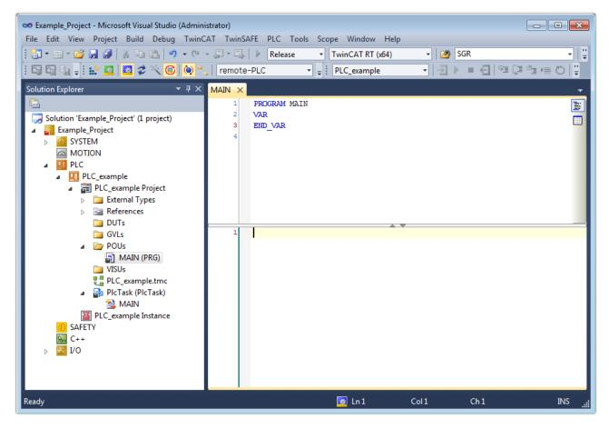
Fig. 78: Initial "Main" program for the standard PLC project
