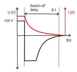
Fig. 17: Switch-off of inductive loads
