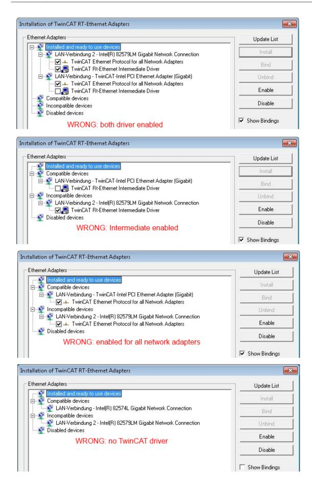
Fig. 97: Incorrect driver settings for the Ethernet port
