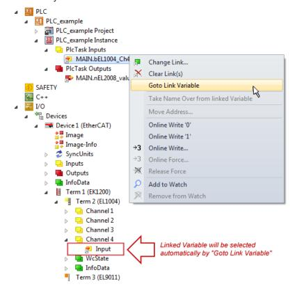
Fig. 84: Application of a "Goto Link Variable", using "MAIN.bEL1004 Ch4" as an example
