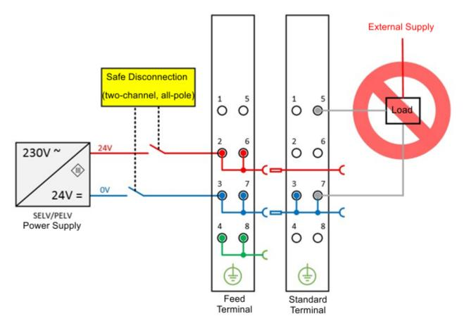
Fig. 4: Negative example - active load
