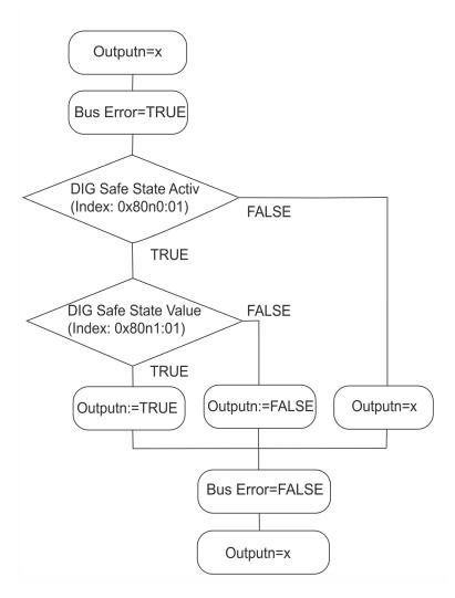
Fig. 22: Change of state of the outputs in the case of a bus error
