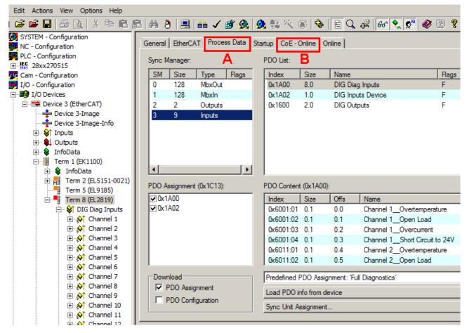
Fig. 18: EL2819 "Process Data" tab
