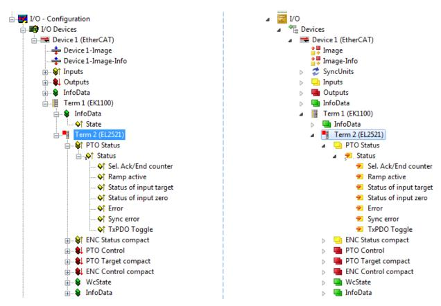
Fig. 116: EtherCAT terminal in the TwinCAT tree (left: TwinCAT 2; right: TwinCAT 3)
