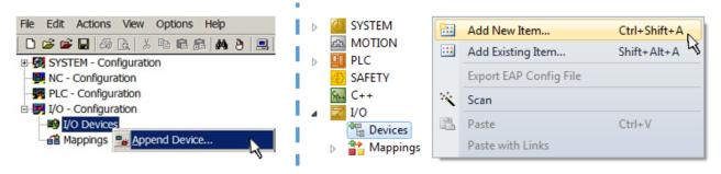
Fig. 107: Append EtherCAT device (left: TwinCAT 2; right: TwinCAT 3)
