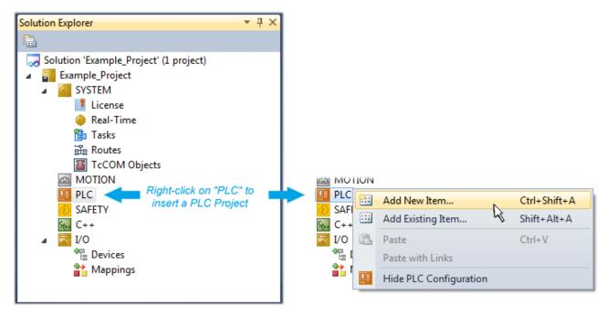
Fig. 76: Adding the programming environment in "PLC"
