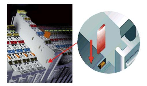
Fig. 39: Power contact on left side
