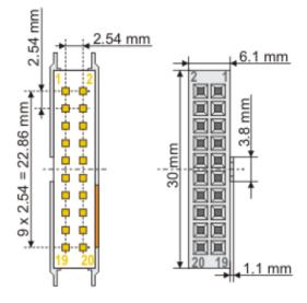
Fig. 26: Dimensions of the 20-pin contact strip of the terminal and the matching spring contact strip; for connections see Contact assignment
