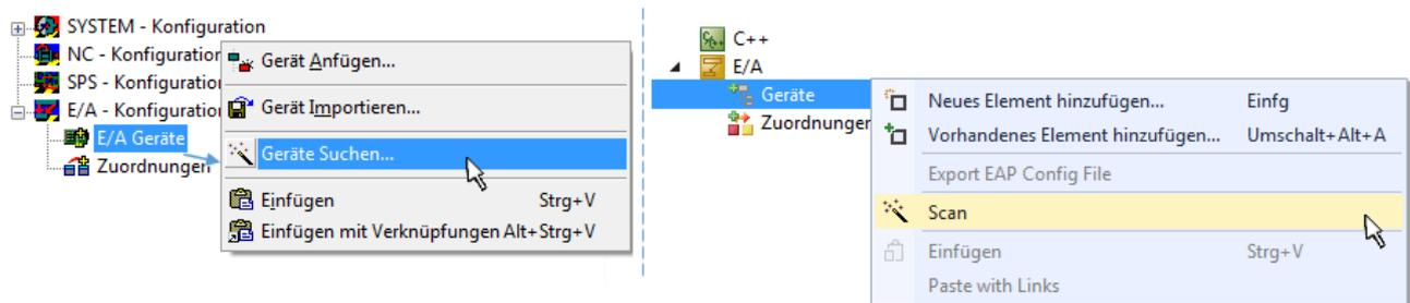
Abb. 118: Scan Devices (links: TwinCAT 2; rechts: TwinCAT 3)
