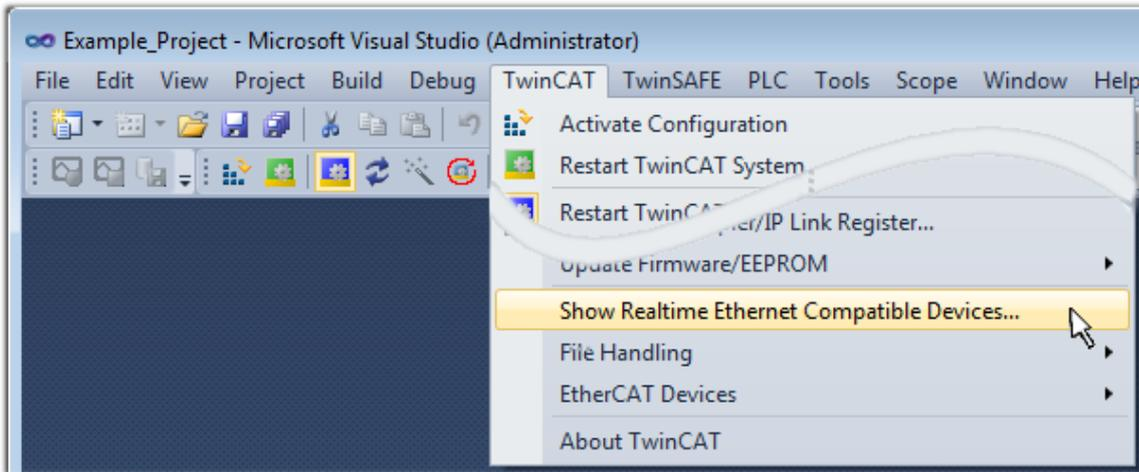
Abb. 91: Aufruf in VS Shell (TwinCAT 3)
