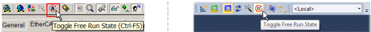
Fig. 137: TwinCAT can also be switched to this state by using a button (left: TwinCAT 2; right: TwinCAT 3)
