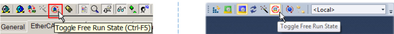
Fig. 102: TwinCAT can also be switched to this state by using a button (left: TwinCAT 2; right: TwinCAT 3)
