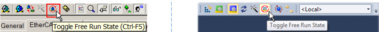
Fig. 103: TwinCAT can also be switched to this state by using a button (left: TwinCAT 2; right: TwinCAT 3)
