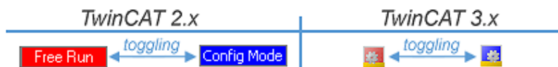
Fig. 105: Displaying of “Free Run” and “Config Mode” toggling right below in the status bar
