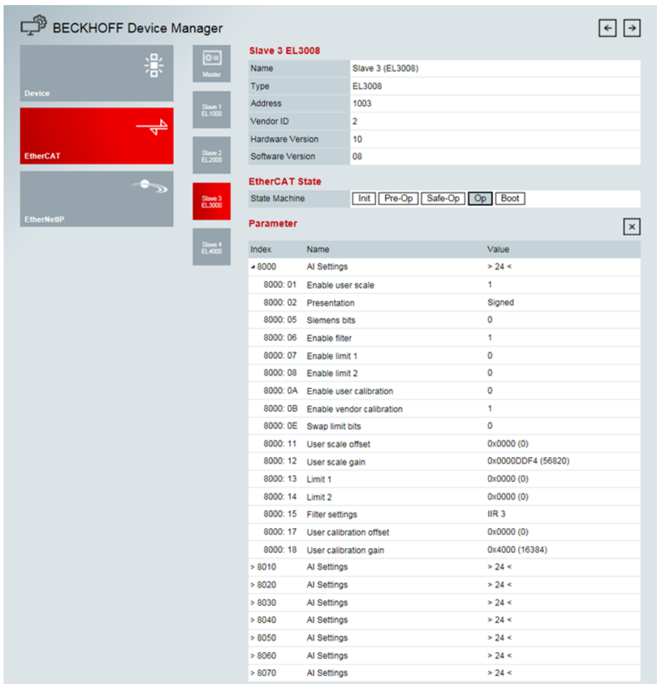
Fig. 20: Configuration via HTML pages - parameterizing EtherCAT Terminals
