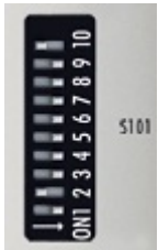
Fig. 15: DIP switch S001: left off "0", right on "1"
