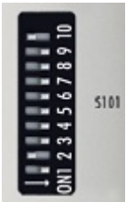
Abb. 15: DIP-Schalter S001: links off "0", rechts on "1"
